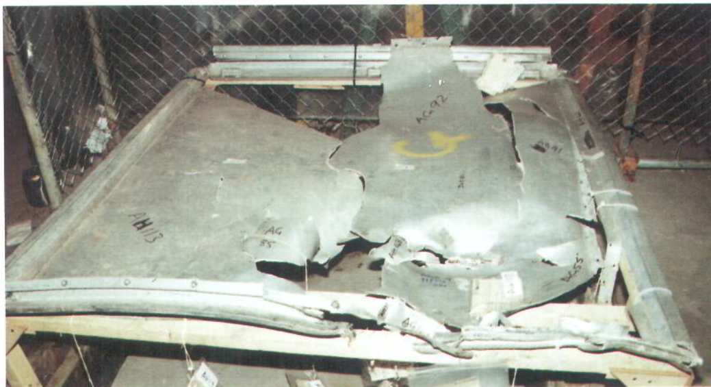
Detail of Damage to Container Floor
