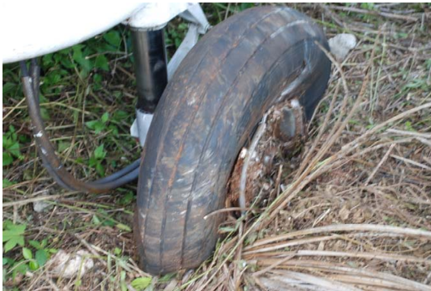
Figure 7: Right Wheel tire and skid mark on it
