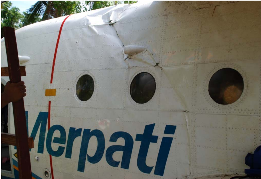
Figure 6: Left side of fuselage wrinkled
