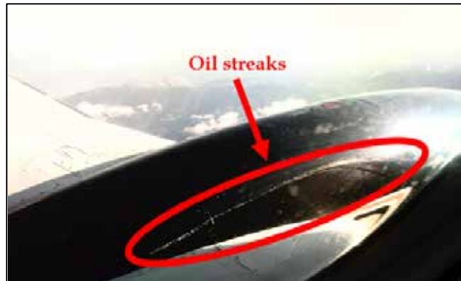
Photo 1. Left-engine oil leak
