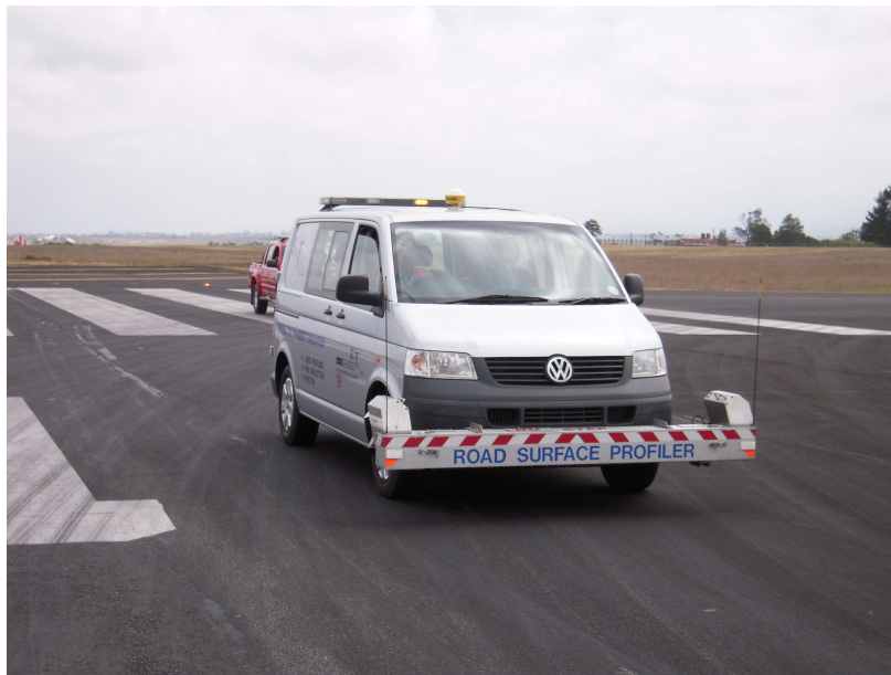
Figure 20: The specialised vehicle used for the Dynatest.
