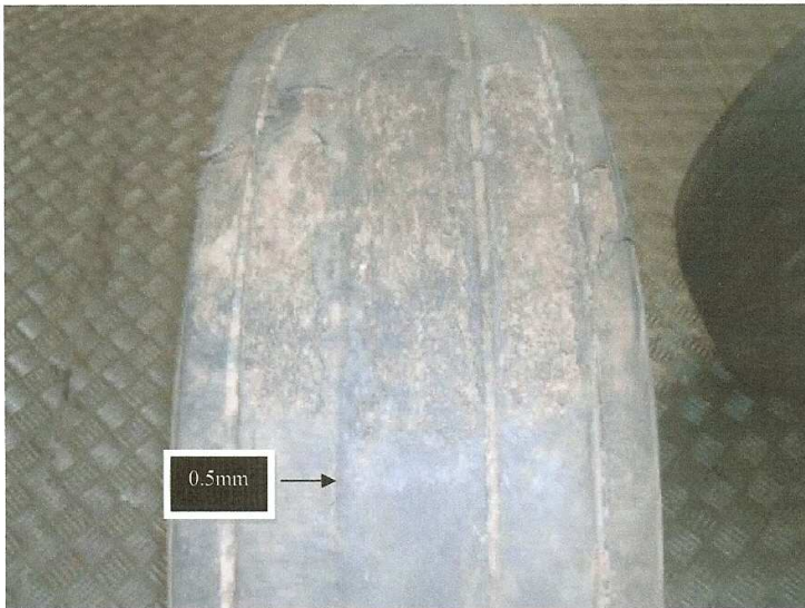
Photo # 1 Tyre serial number 08284318 exhibiting an area of tread with partial melting of tread rubber approximately the area of the tread footprint.
