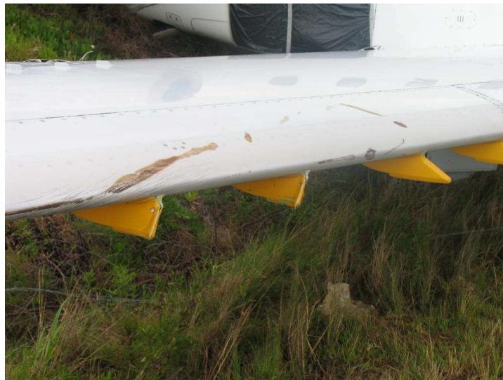
Figure 40(a): Damage to the right wing leading edge.
