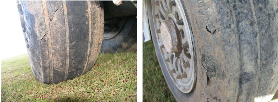
Figure 43: The two tyres on the left main gear assembly showed evidence of hydroplaning and side impact damage.
