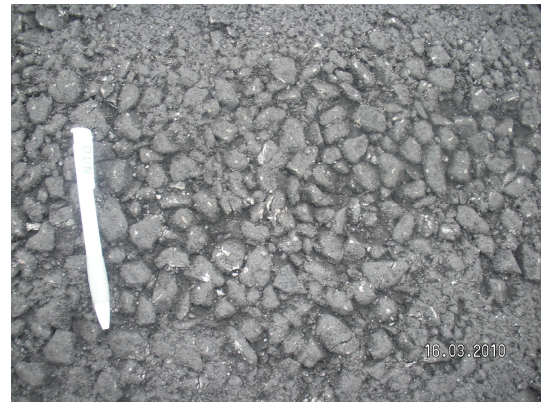
Figure 23(b): Close-up of the milled aggregate, which was 15-20 mm in diameter.
