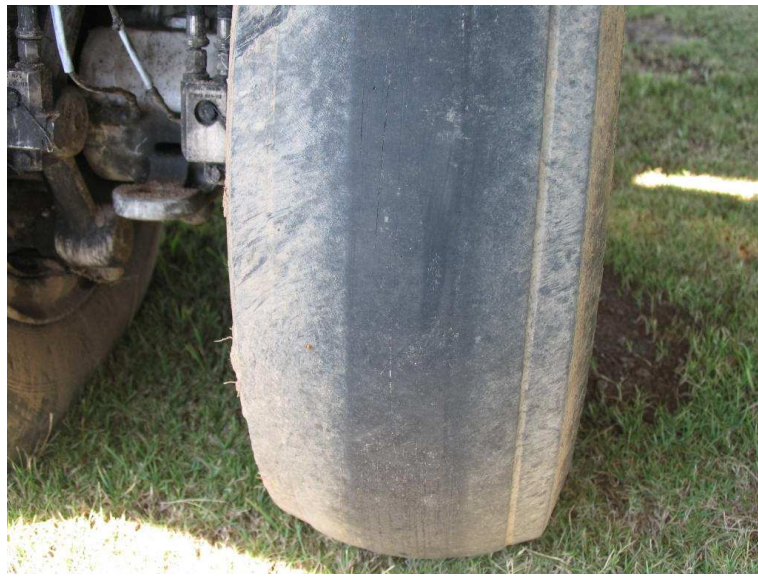
Figure 45: The tread of the left main inner tyre showed an advanced state of wear.
