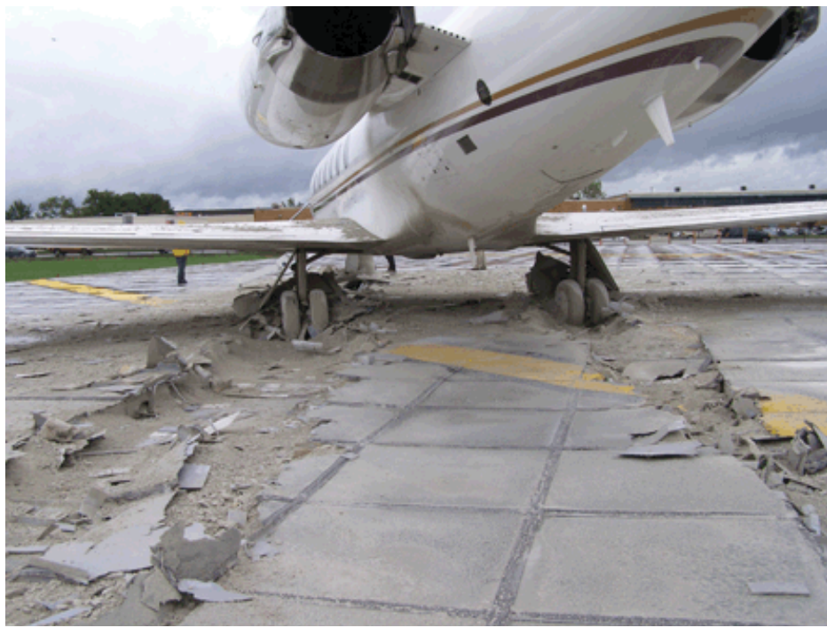
Figure 56: A Cessna Citation 550 that overran the runway at Key West International Airport, Florida, USA. Note the crushable concrete blocks.
