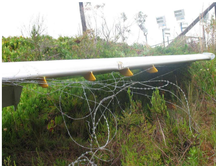
Figure 40(b): Damage to the left wing leading edge.
