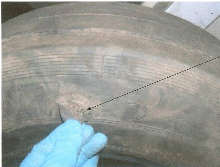
Photo # 2 tyre serial number 08284318 shows gouges and cuts to the tyres sidewall. This damage is considered to have occurred as a result of the tyre aquaplaning
