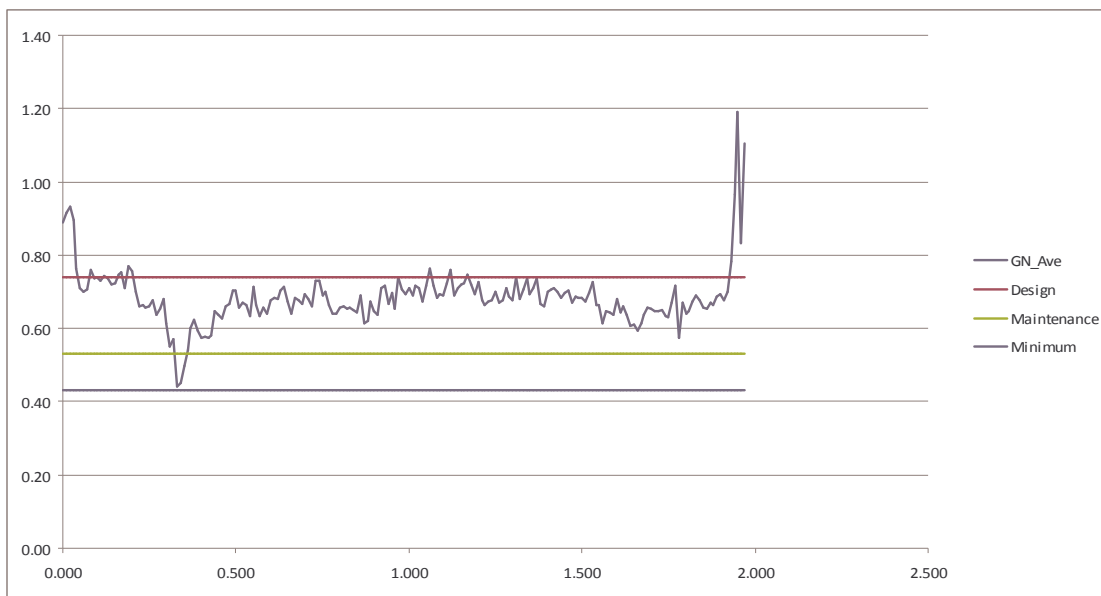
Figure 16(a): Friction test result for runway 29 – taken one metre to the left of the centreline.
