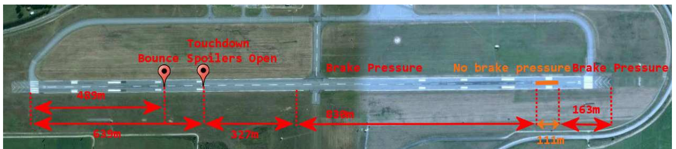
Figure 33: The landing sequence of the aircraft. Distances are estimates, based on DFDR data.
