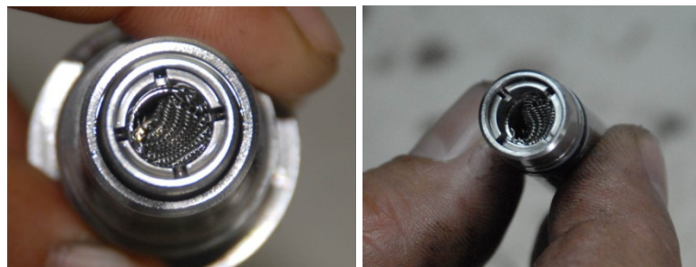
Figure 12: Left restrictor check valve screen damage, up flow direction
