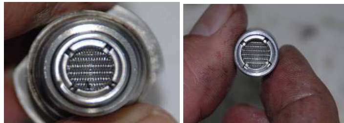
Figure 13: Left restrictor check valve, the opposite screen still intact, down flow direction
