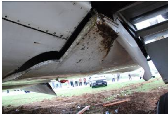
Figure 2: Left main landing gear door
