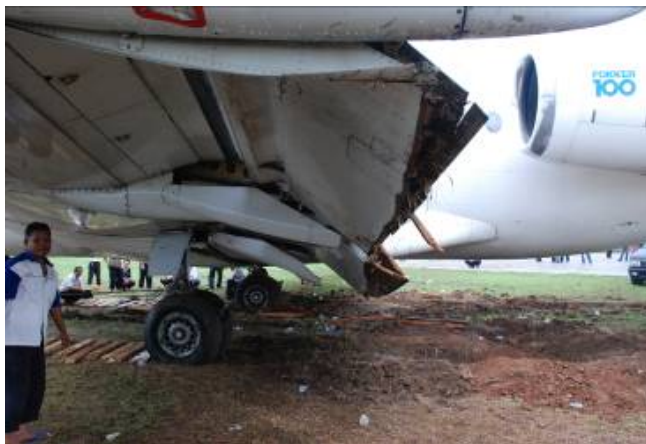
Figure 3: Inner and outer flaps were damage
