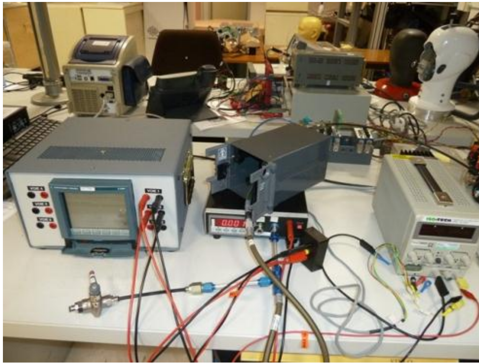
Figure 66 : Photo of MXP147-3 pressure switch actuation test set-up
