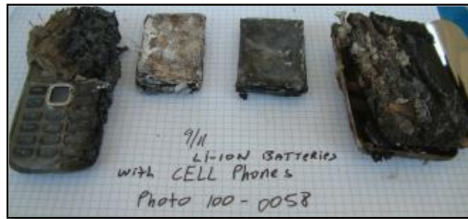
Intact and fire damaged Panasonic batteries (2-pack Li-ION set)[LH]/Mobile phones and batteries [RH]
