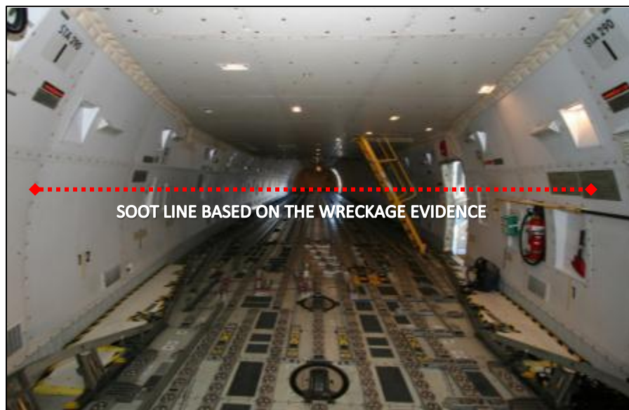
Photo 17 Exemplar interior showing stairs to the flight deck and a dotted line showing the level of the smoke layer
