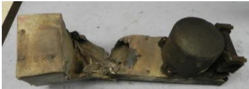
Picture 3 Damaged Flight Data Recorder in the Recovered condition
