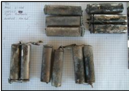
Additional battery pack remains [LH]/D-Cell size lithium primary batteries. Photo shows fire damaged and undamaged batteries [RH]
