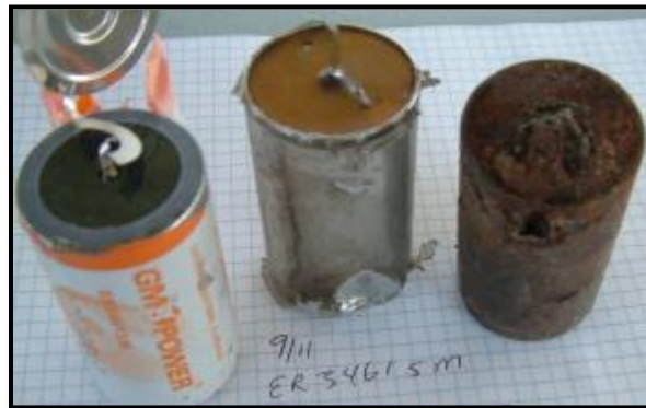
Additional battery pack remains [LH]/D-Cell size lithium primary batteries. Photo shows fire damaged and undamaged batteries [RH]
