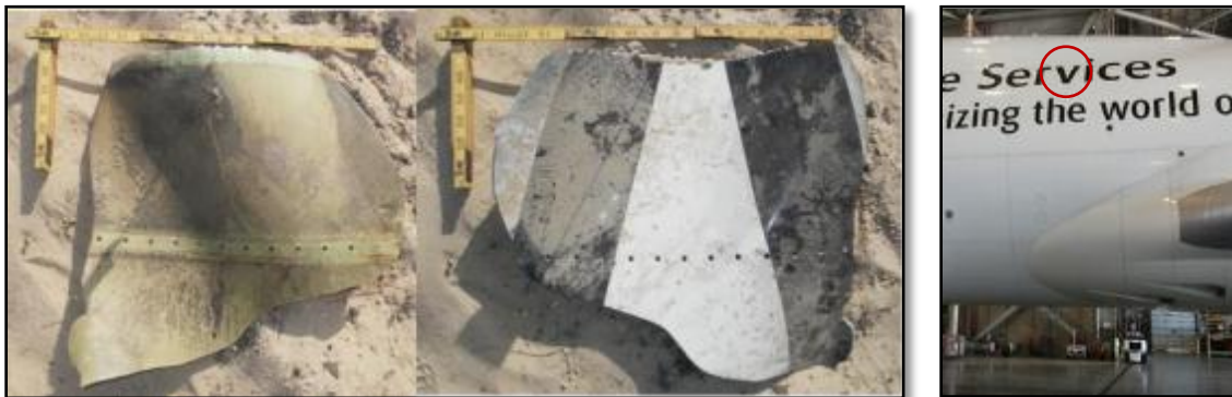
Photo 7 Recovered Fuselage skin section [LH]. Exemplar aircraft exterior [RH]
