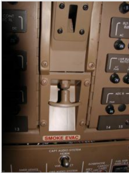
Figure 99: Smoke Evacuation Handle Figure 100: Smoke Evacuation Port (cockpit ceiling)
