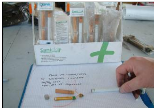
Electronic cigarettes containing lithium primary batteries 55
