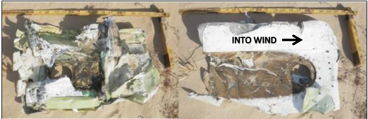
Photo 10 Fuselage skin piece with smoke shutter cut-out (interior on the left, exterior on the right)
