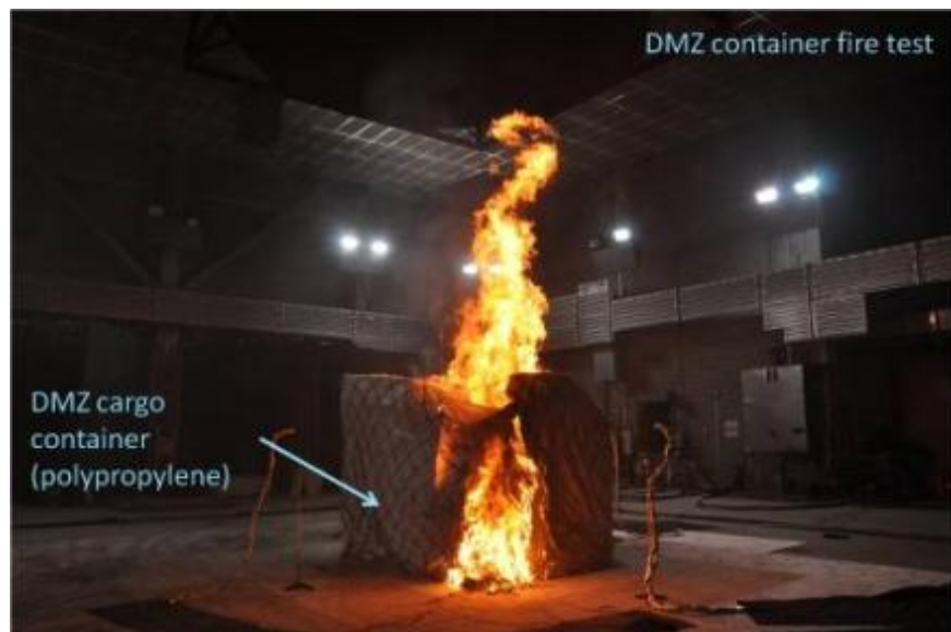
Photo 2 - NTSB DMZ Cargo Container fire depicting a polypropylene cargo container burning at a rate of 8.45MW, 132 seconds after becoming detectable to an aircraft-based smoke detection system.
