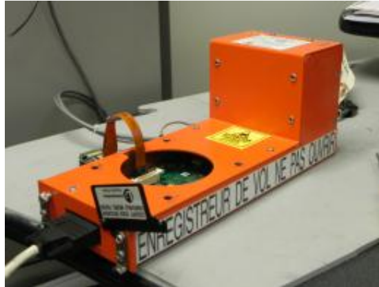
Picture 4 – The FDR Memory Connected to the Surrogate Recorder
