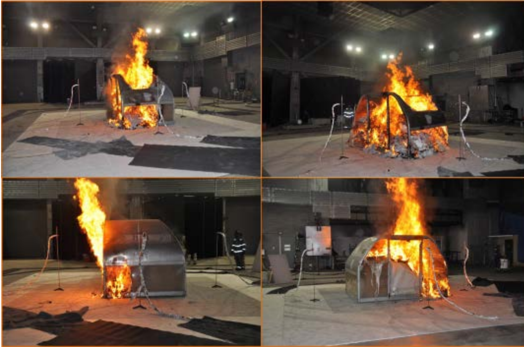
Figure 29 A2N Cargo Container Fully Developed Fire
