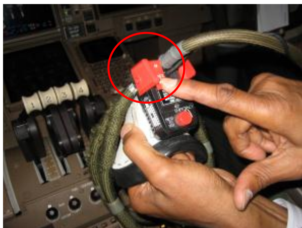
Figure 106: 100% Selector Switch on Oxygen Mask
