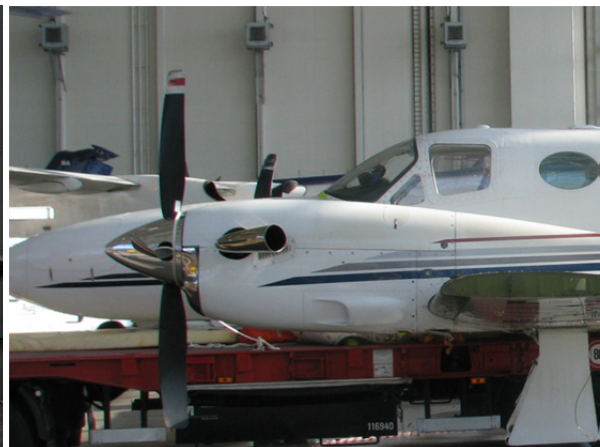
Position and deformation of the propeller blades of the left engine at the accident site and after the salvage operation and the transport to a hangar
