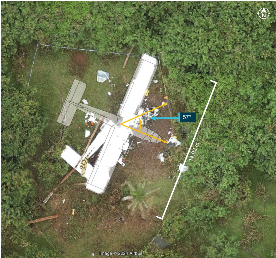
Figure 8: Accident site showing position of YJ-AT2 and rotation of fuselage about wings
