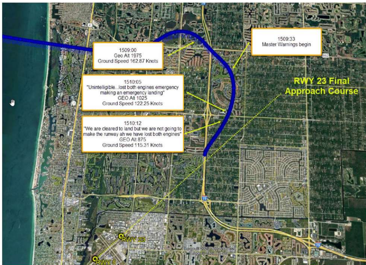
Figure 1. ADS-B ground track (blue dots) with annotations of specific events during the approach, including time and the airplane's geometric altitude and ground speed (source: FAA).
