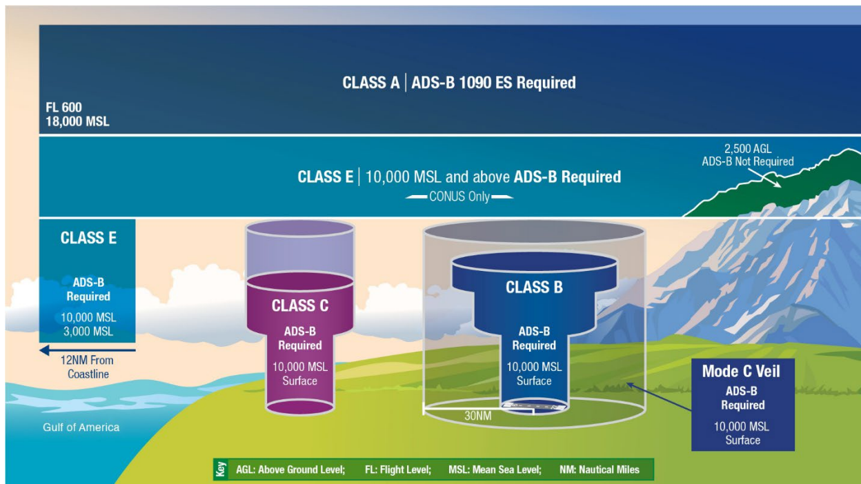
Figure 9. ADS-B Out equipage mandates in the NAS, by categories of airspace. (Source: FAA)
