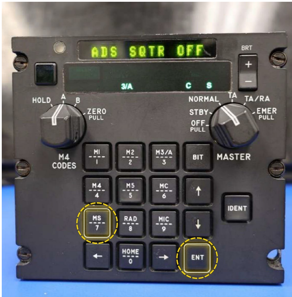
Figure 5. A UH-60L transponder with the ADS-B squitter turned off. (Source: BAE Systems)
