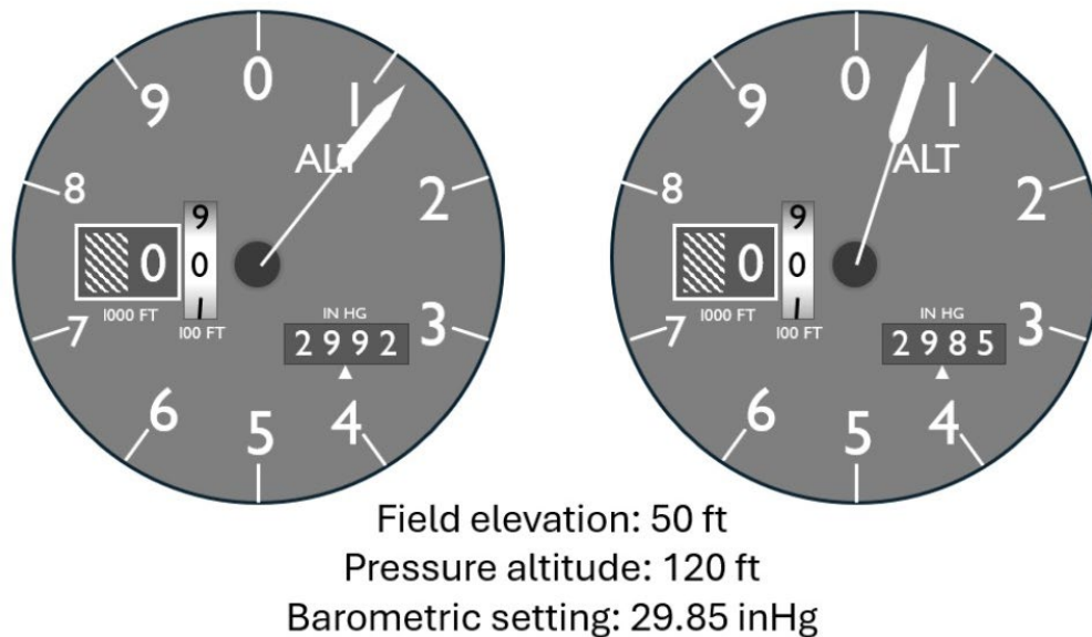
Figure 40. Comparison between pressure altitude and corrected barometric altitude.
