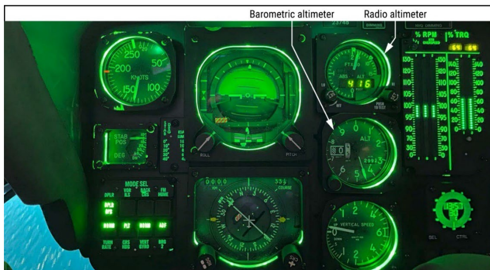
Figure 7. Photograph of the instrument panel on the left side of a UH-60L cockpit, as viewed when looking below NVGs.
