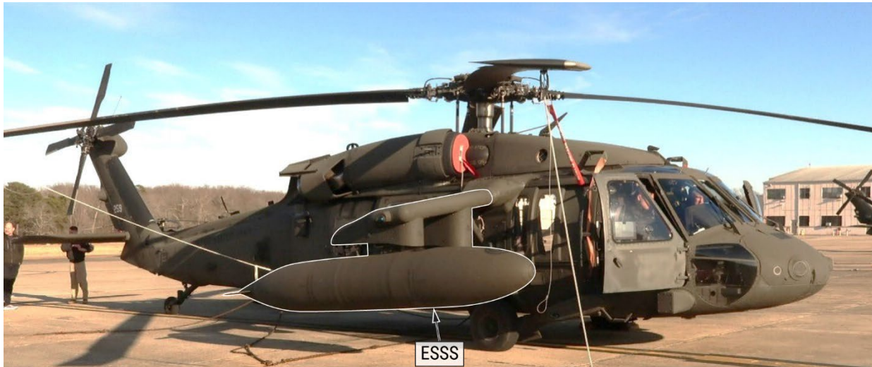
Figure 4. Photograph of exemplar 12th Aviation Battalion UH-60L equipped with ESSS and external fuel tanks.
