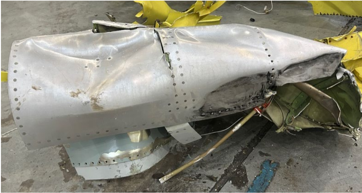
Figure 29. Wide view of impact mark on the airplane's left wing inboard leading edge slat.
