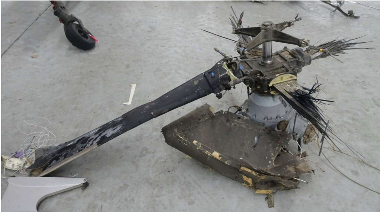
Figure 32. The helicopter's tail rotor as recovered, attached to the tail rotor gearbox.
