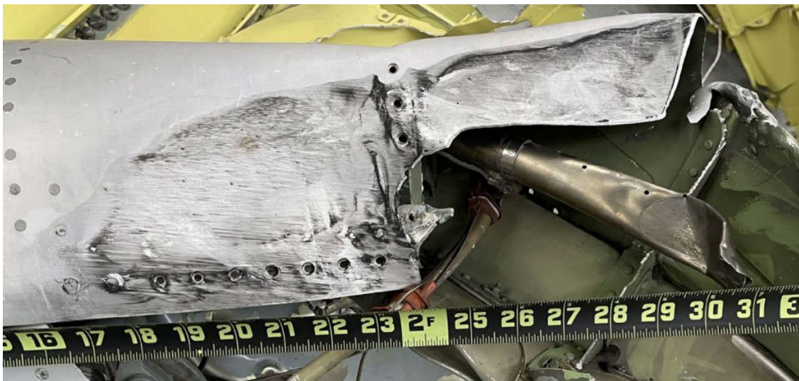
Figure 30. Close-up view of impact mark on the airplane's left wing inboard leading edge slat.
