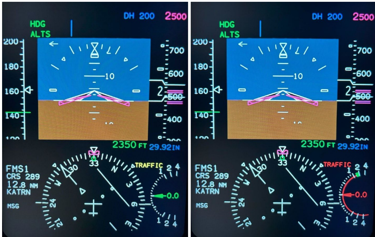
Figure 10. PFD depicting an active traffic advisory (TA) shown on left, and an active resolution advisory (RA) shown on right.
