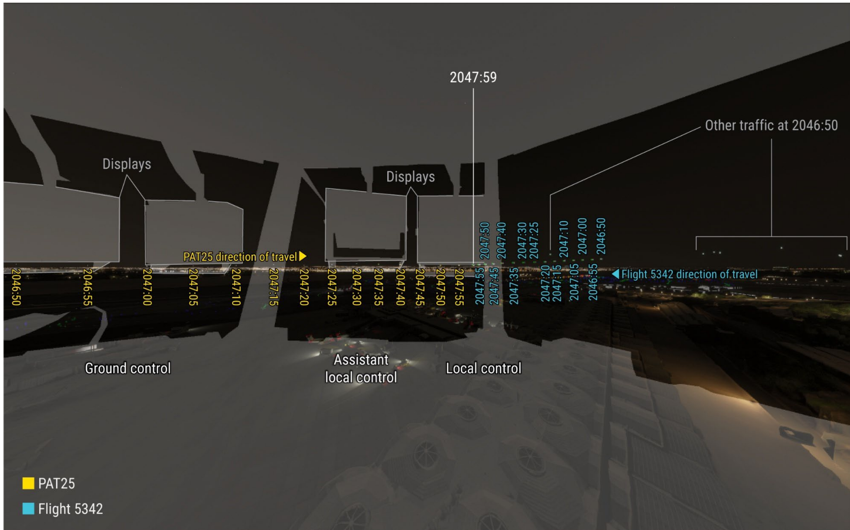
Figure 60. Simulation of the views from the ATC tower cab of the helicopter and airplane during the approximate minute before the accident, with aircraft positions at the labeled times.
