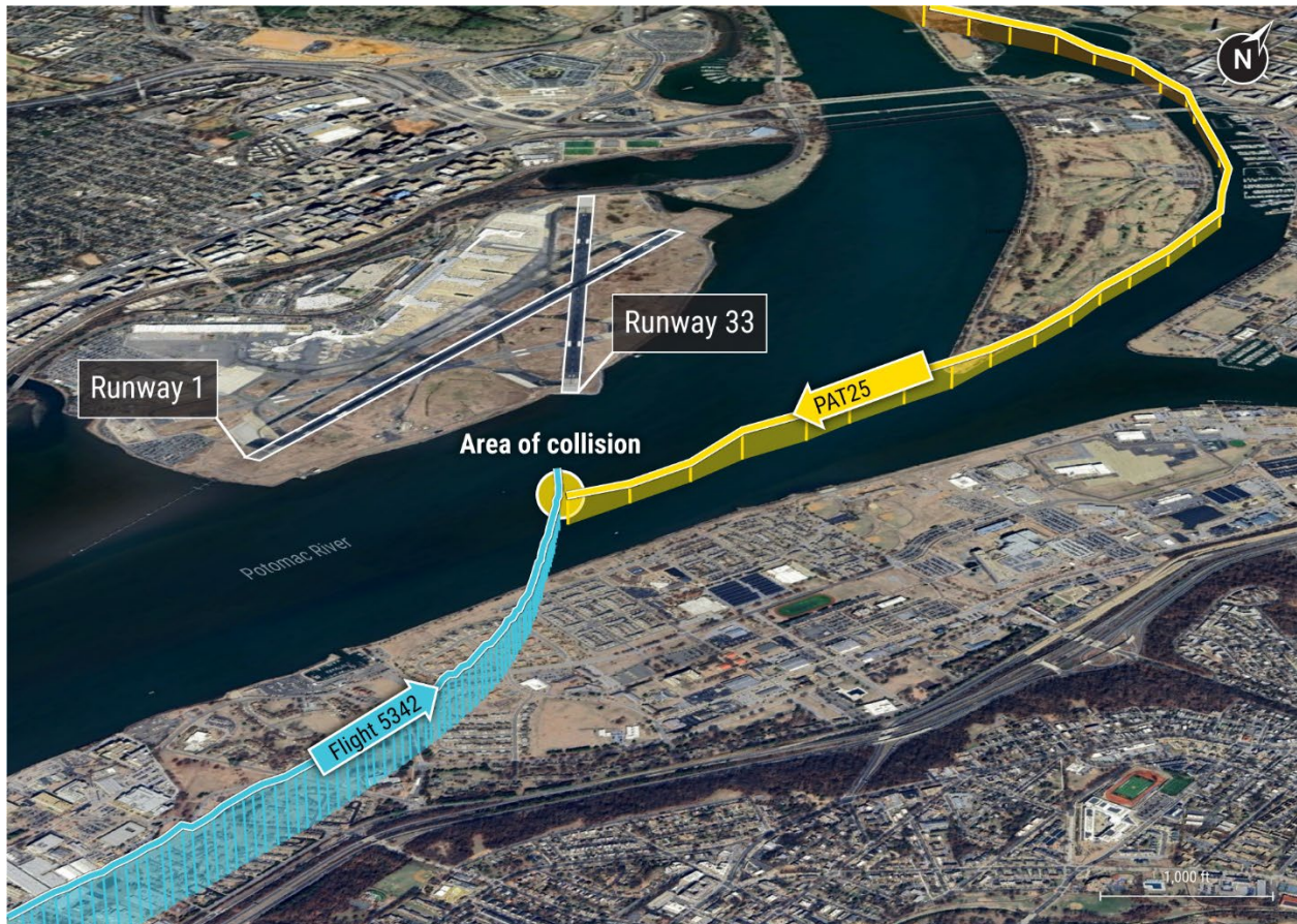
Figure 3. Oblique aerial illustration of the Automatic Dependent Surveillance–Broadcast flight track for flight 5342 (yellow line) and the composite data-derived flight path for PAT25 (blue line) converging near DCA.
