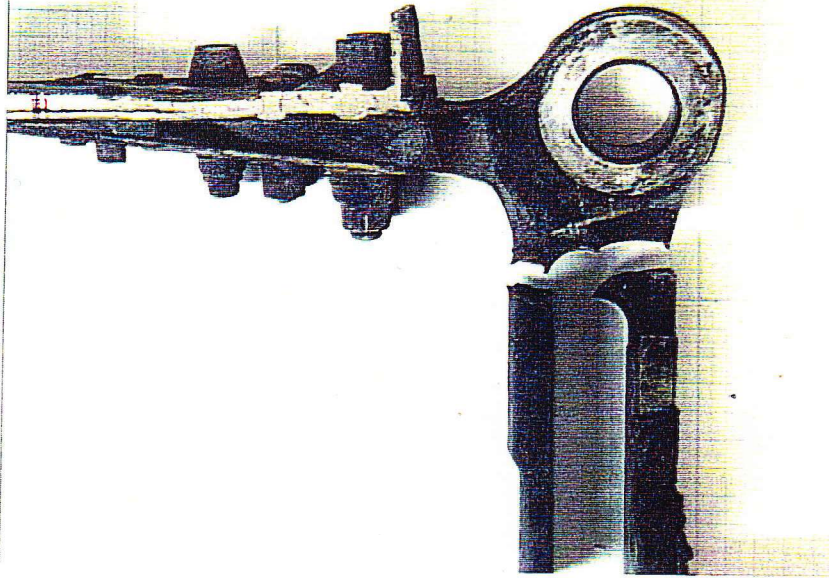
Picture 9: Mating part of the fitting removed from aircraft relative to the disassembled fractured upper and lower tangs.
