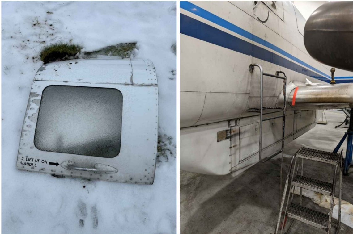
Figure 1. Cockpit hatch as found. Figure 2. Exemplar ladder and hatch above.
