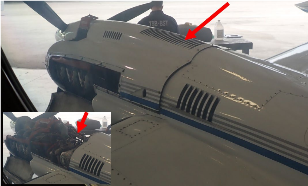
Figure 3. Approximate location of the in-flight fire indicated by arrows, with inset image showing the approximate fire location with the upper engine cowling removed. The pictured aircraft is a Cessna 421B, which has the same engine and nacelle as the Cessna 421C (Source of main image and inset: TSB)
