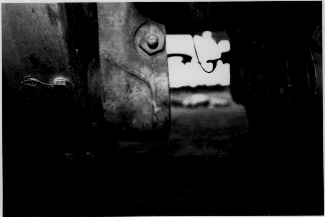
Right Main Gear Outboard Brake Caliper Showing New Gouging on Front Figure 27
