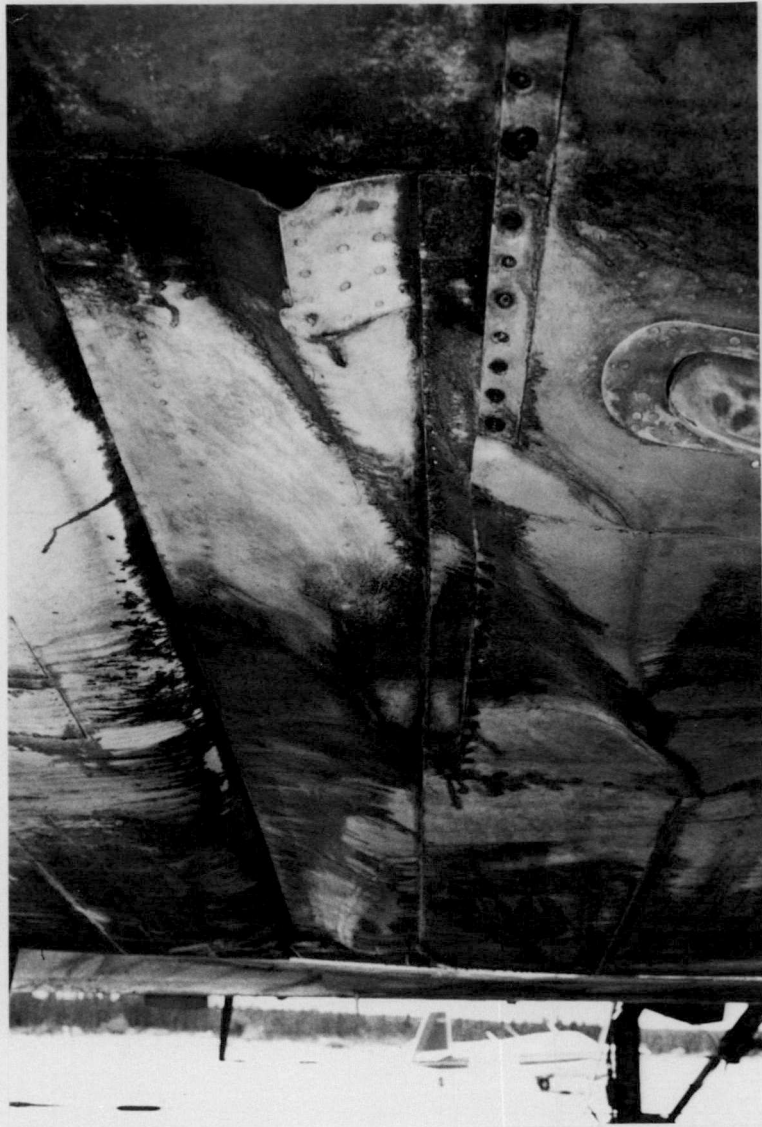
Close-up of Damage to Right Wing Undersurface and Flap Fairing
