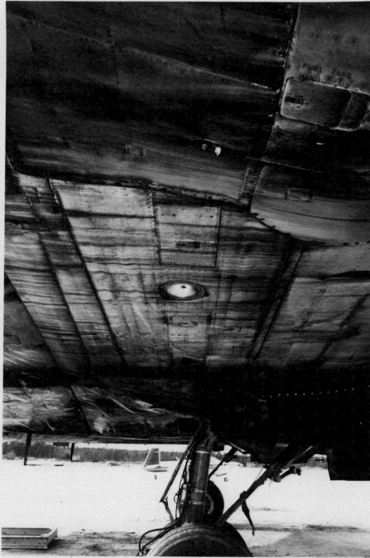
Right Main Gear Exhibiting Rearwards Inclination
