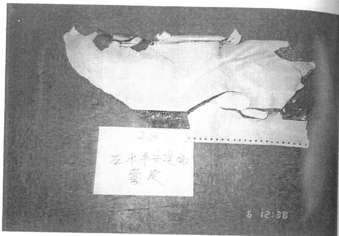
28. SKIN OF LH HORIZONTAL STABILIZER 左水平安定面蒙皮
