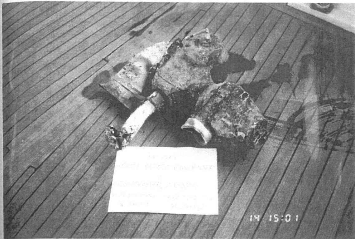
56. DUCT OUTLET CONDENSER (P/N:782274-1, S/N:920315) & CONDENSER MIXER (P/N:776916-2, S/N:920817) 凝結器導管及凝結器本體
