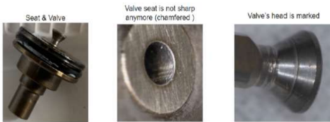
Figure 36 - Damage in the seat and valve
