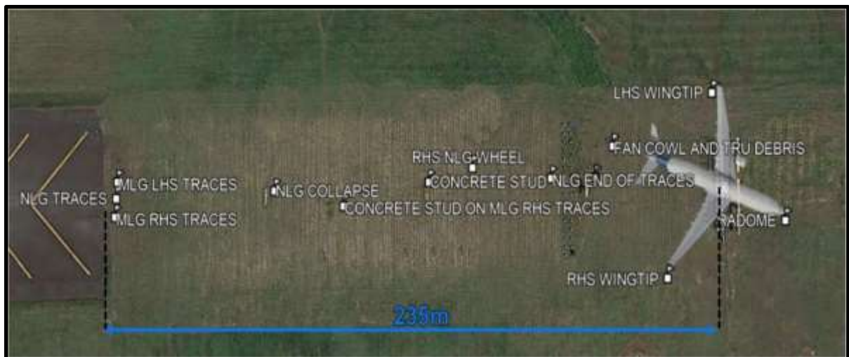
Figure 5 - The aircraft path exiting RWY 22.
