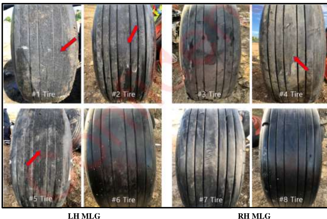
Figure 31 - Tire condition after the accident as per Airbus wheel numbering convention.
