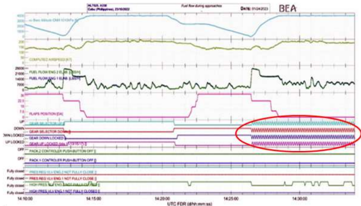
Figure 25 - Landing gears undetermined position.
