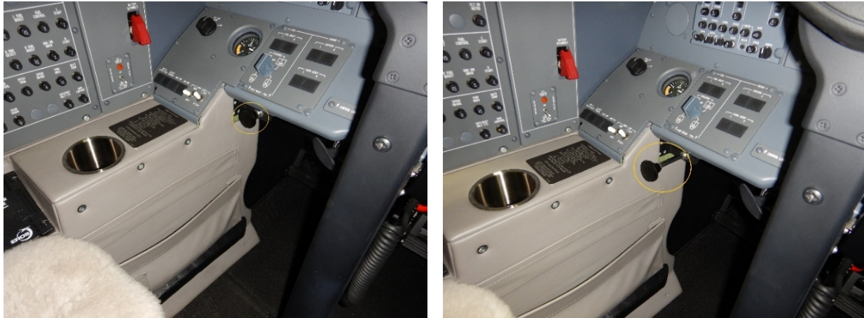
Figure 1. Pictures from an exemplar 560 XLS+ showing the parking brake off (left) and set (right).
