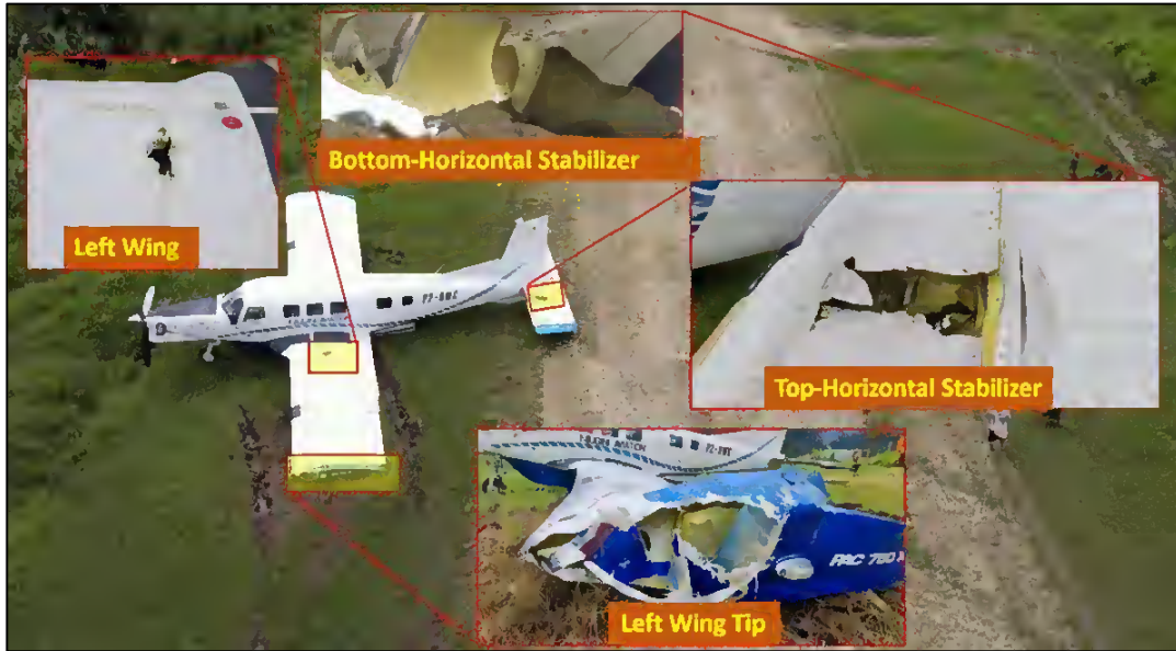
Figure 11. Damage to the aircraft structure.
