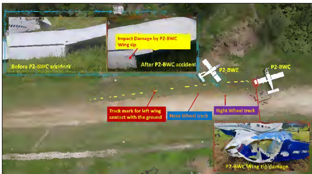
Figure 3. Damage caused to P2-BWE by P2-BWC.
