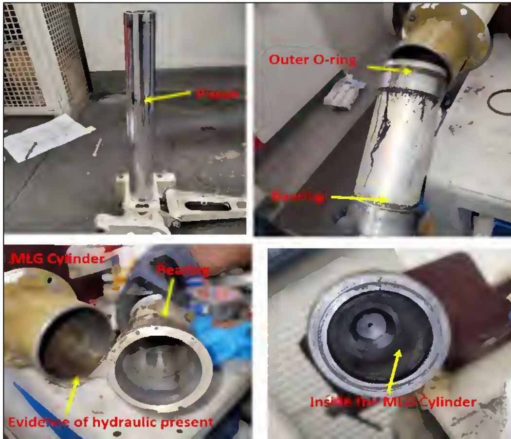
Figure 16. Observations on the MLG oleo strut.
