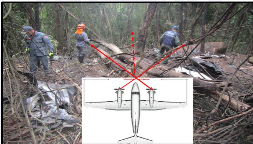
Figure 8 - Impacted tree, aircraft trajectory and final position of the engines.
