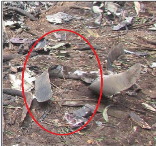
Figure 13 - Image of one of the propeller sets. In the red highlight, one of its blades deformed in the direction of flight.
