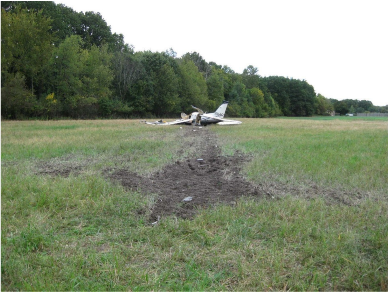
Figure 5. Initial impact point and ground scar.
