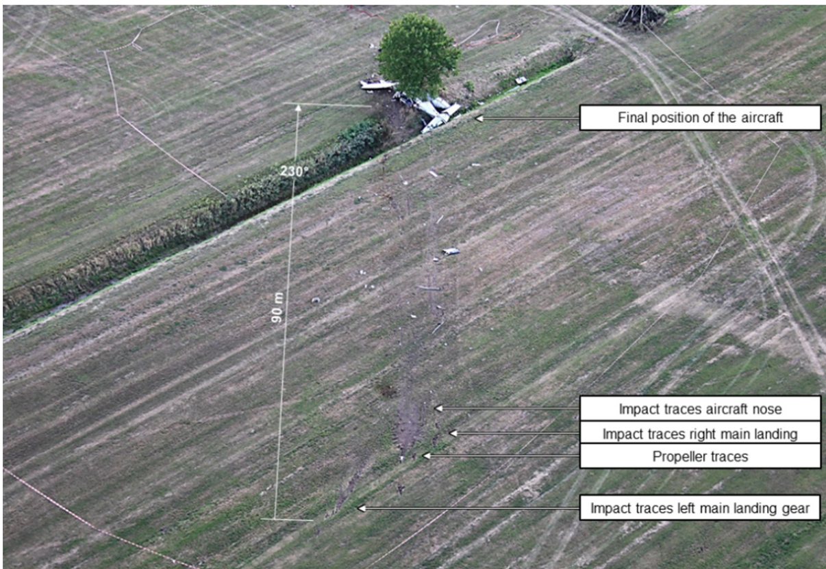
Fig. 7: Ground traces at the accident site
