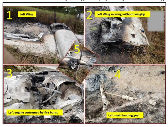
Figure 4: Damage to left wing
