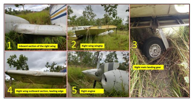
Figure 5: Damage on the right wing
