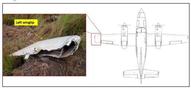
Figure 3: Damage to left wingtip
