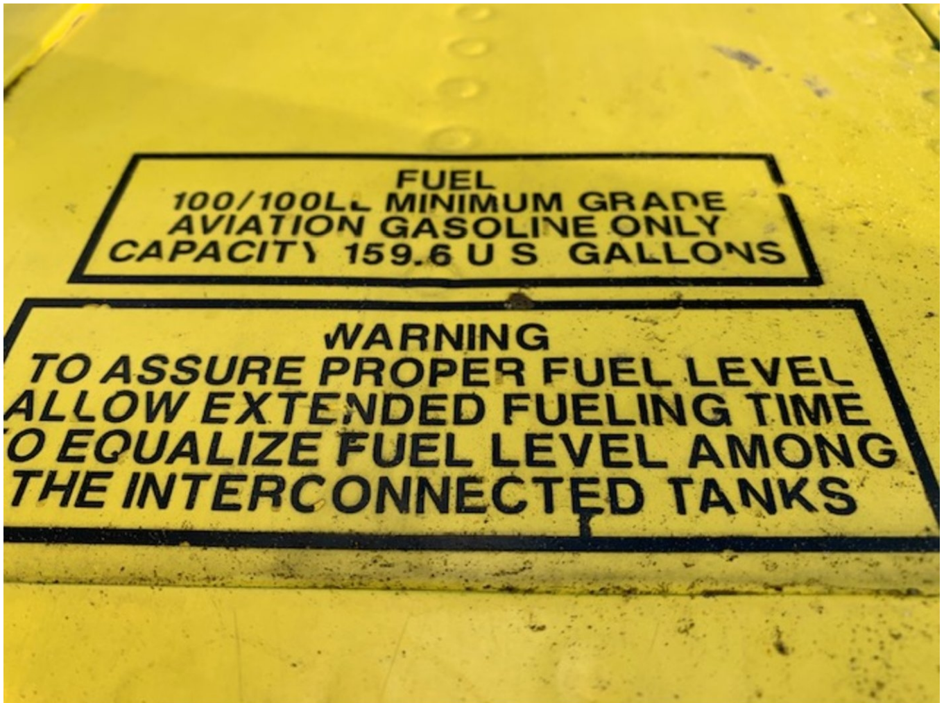
Figure 1 - Fuel placard on accident airplane located near fueling port.
