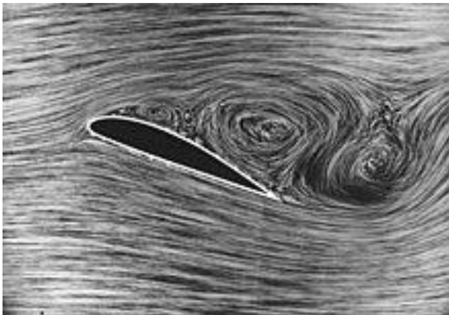
Figure 12: Picture showing Airflow separating from an aerofoil at a high angle of attack, as occurs during stall.
