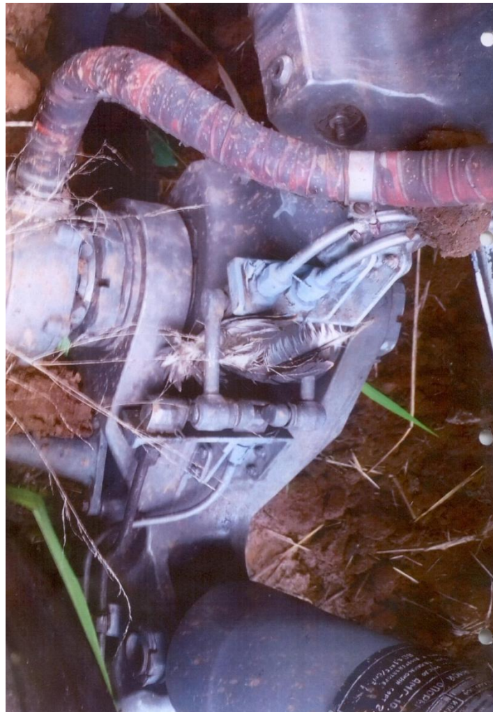
Figure 21: Picture showing the bird remains entangled in the nose wheel.
