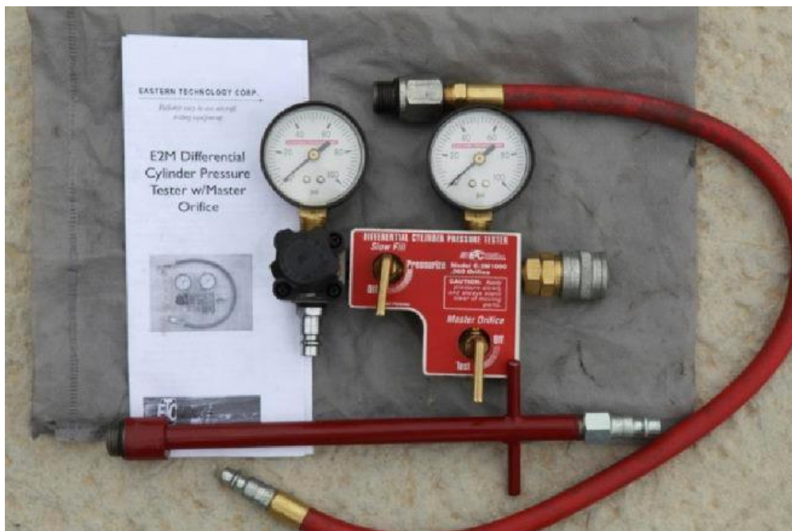
Рис. 21. Тестер Differential Cylinder Pressure Tester E-2M1000.060
