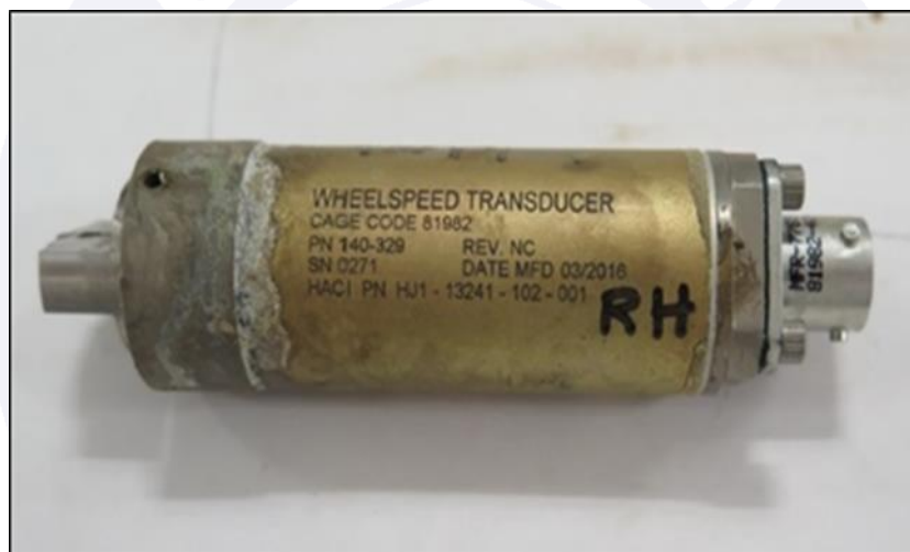
Figure 6 - View of the Wheel Speed Transducer (WST) from the aircraft's right wheel.
