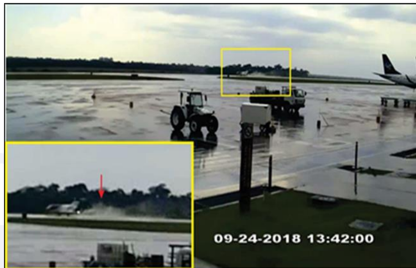
Figure 20 - Detail of the landing run, highlighting the spray formed on the back of the aircraft.
