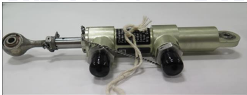
Figure 2 - View of one of the four master cylinders installed on the aircraft.
