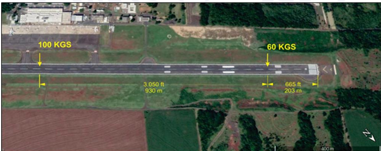
Figure 35 - Representation of the distance traveled by the aircraft from the point of 100 KGS to 60 KGS.
