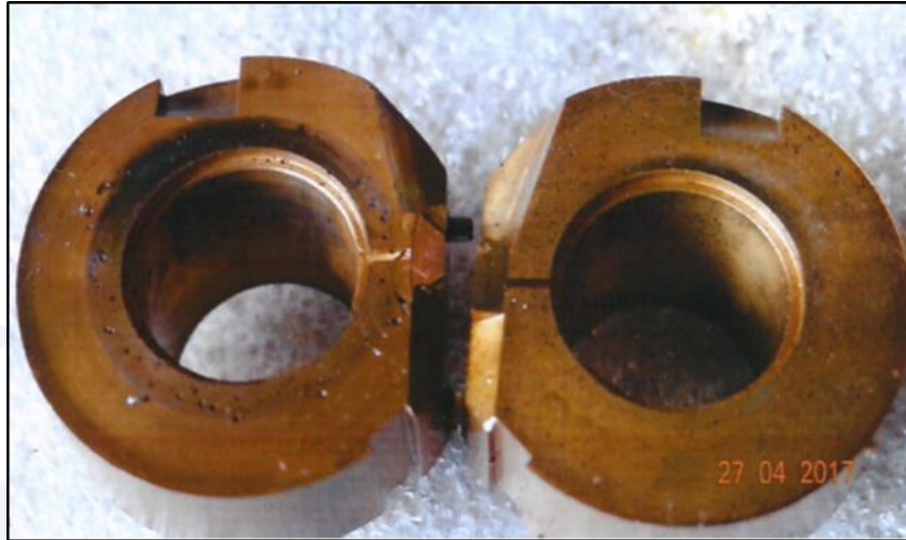
Figure 5 - View of left engine fuel pump bushings with evidence of cavitation.
