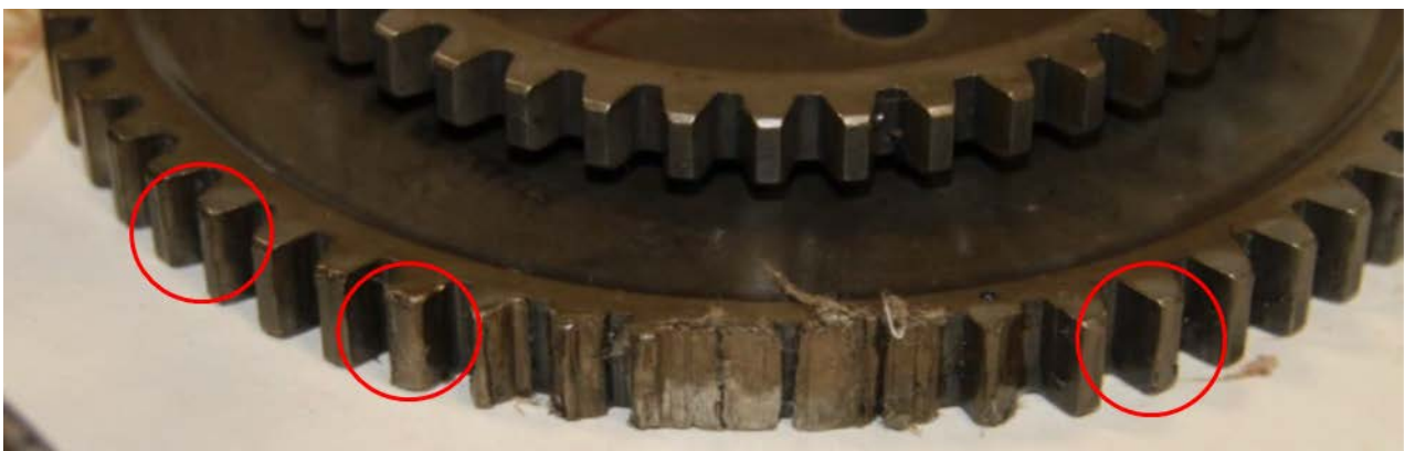
Fig. 6.1: Damaged faces of teeth on L2 gear
