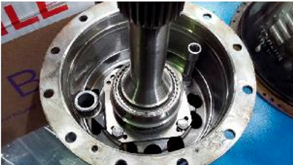
Illustration 16: Close-up of gear box, showing only two of the four bolts
