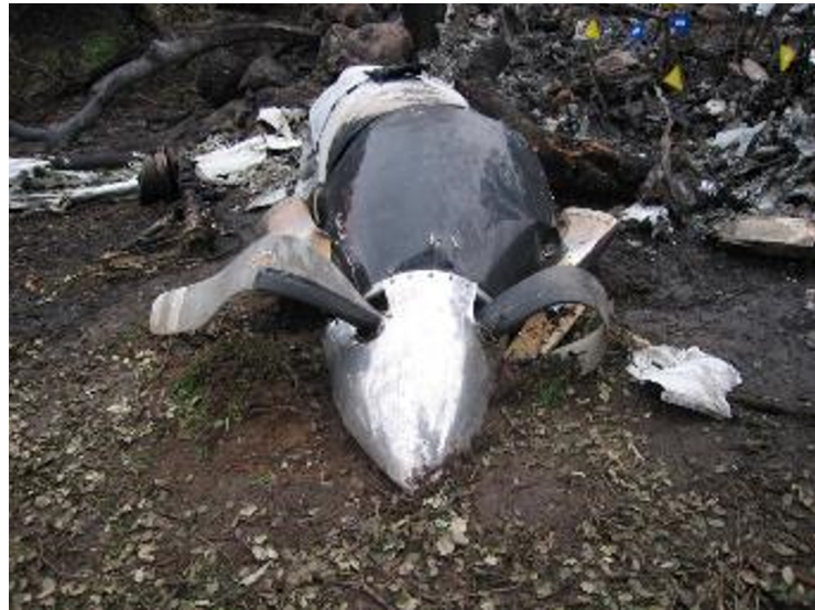
Illustration 14: Right engine at the crash site
