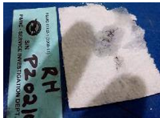
Illustration 15. Close-up of metal particles found in the chip detector in the right engine
