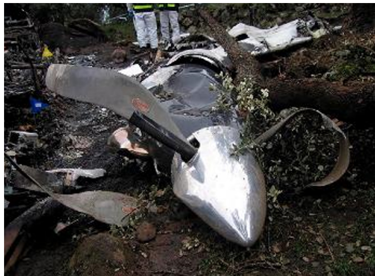
Illustration 13. Left engine at the crash site
