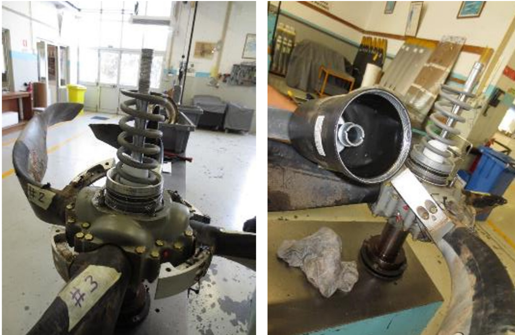
Illustration 18: Close-up of the spring and cylinder on the left propeller
