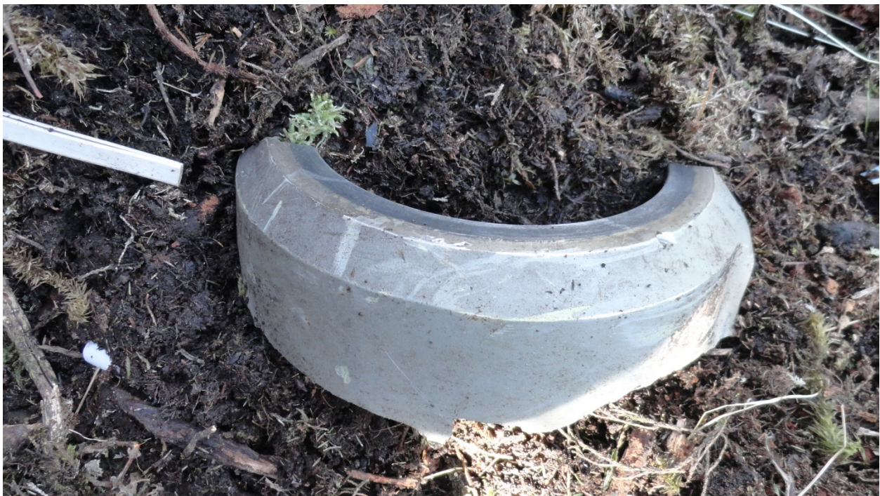
Figure 7: The severed and sheared portion of the bulkhead
