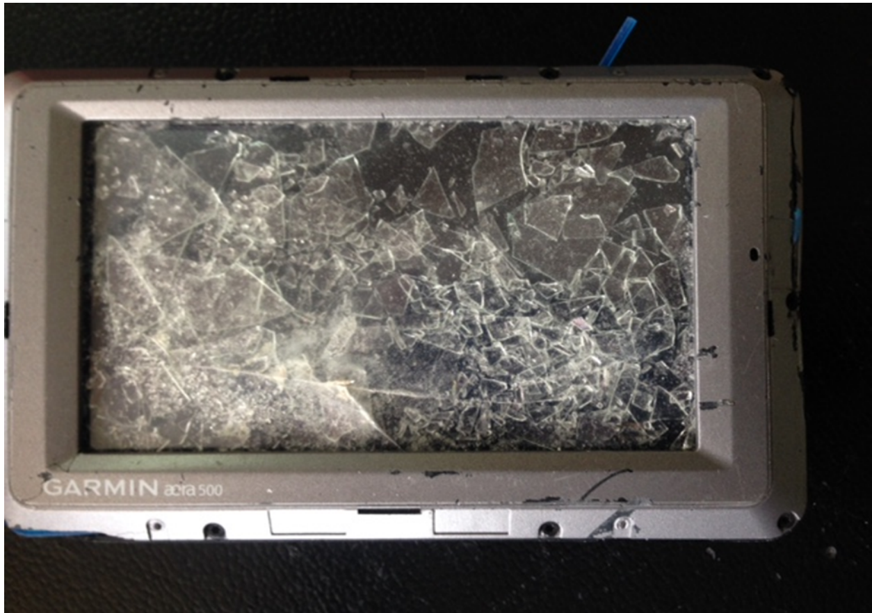
Figure 14: The GPS Garmin Aera 500 after recovery from the wreckage
