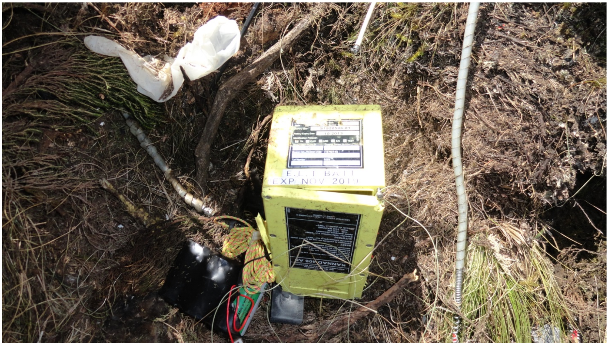
Figure 12: The ELT with the batteries still attached at the accident site
