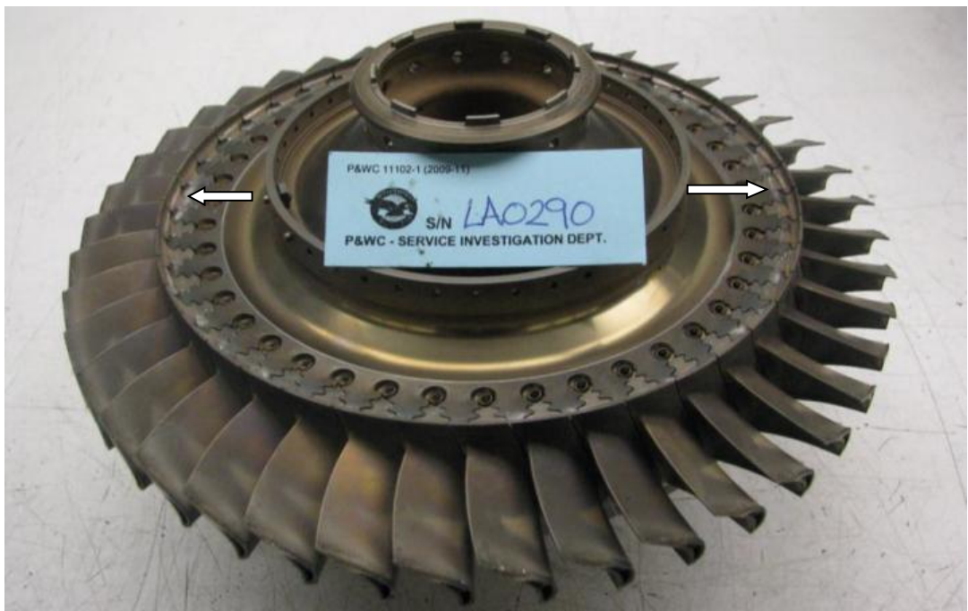
Figure 31: The high-pressure turbine disk (trailing edge view), with some rub marks visible
