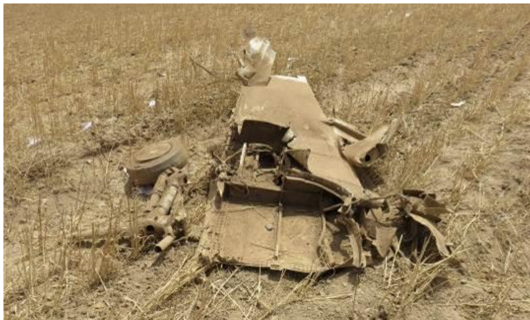
Figure 11: The inner section of the left wing and the left main gear
