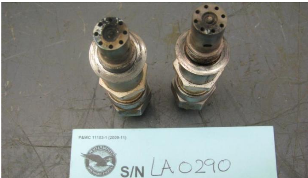
Figure 33: The ignitor plug faces were not damaged, but they display some carbon accumulation
