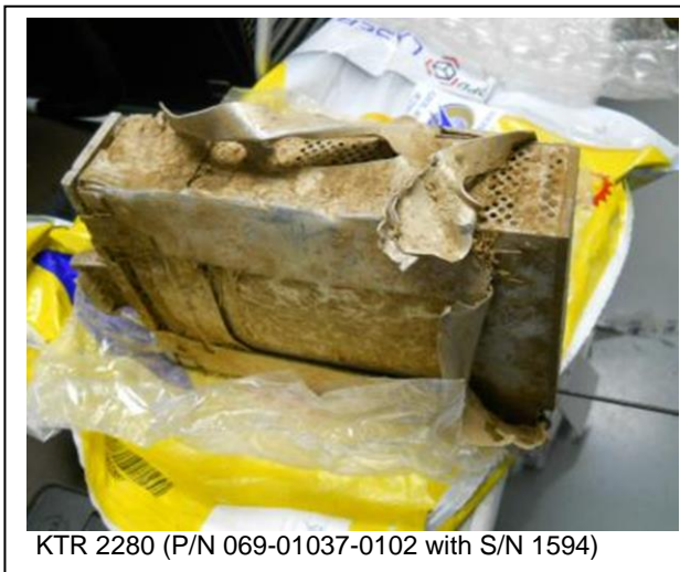
Figure 18 and 19: The KTR 2280 and EGPWS units that were sent to the USA for downloading
