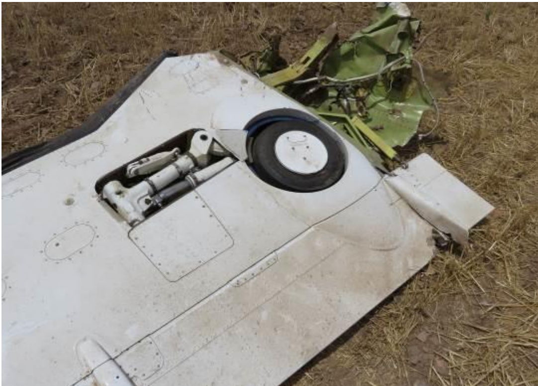
Figure 13: The right wing with the main gear still in the retracted position
