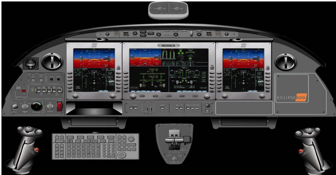
Figure 5: The AVIO NG glass cockpit fitted on the Eclipse aircraft
