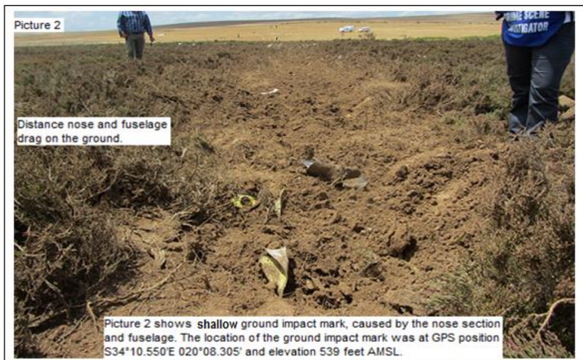
Figure 7: The ground impact mark of the nose and fuselage
