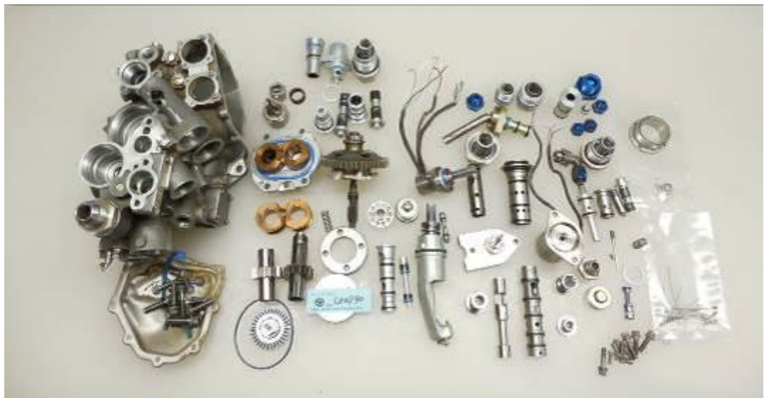
Figure 35: The fuel metering unit after it was dismantled
