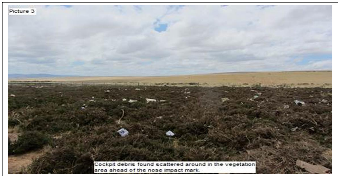
Figure 8: Scattered debris from the cockpit and cabin area ahead of the nose impact mark
