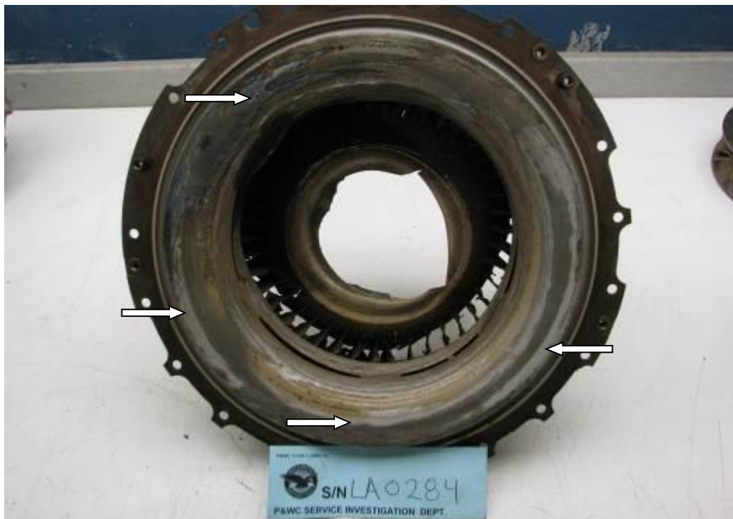
Figure 24: Rub marks on the No. 1 engine centrifugal compressor shroud
