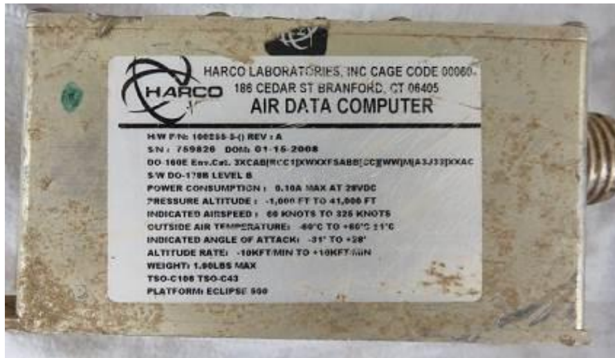
Figure 38 The air data computer that was recovered
