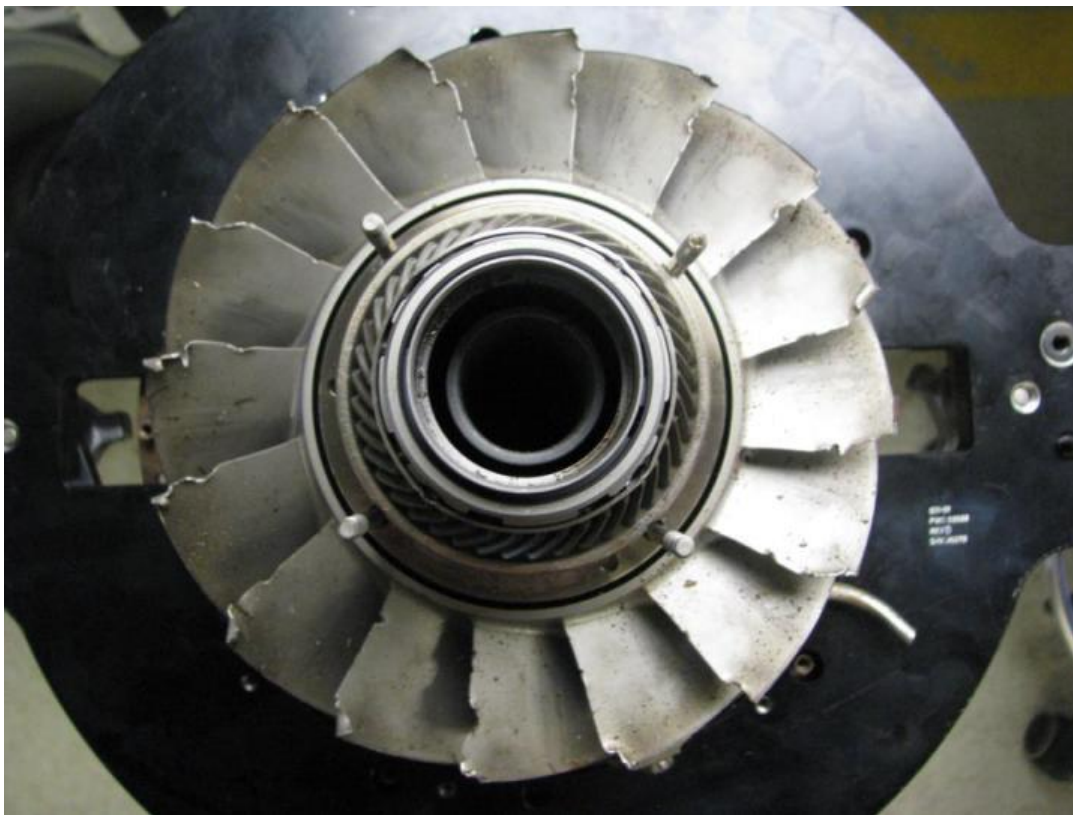
Figure 27: Damage to the axial compressor (No. 2 engine) associated with debris impact during rotation
