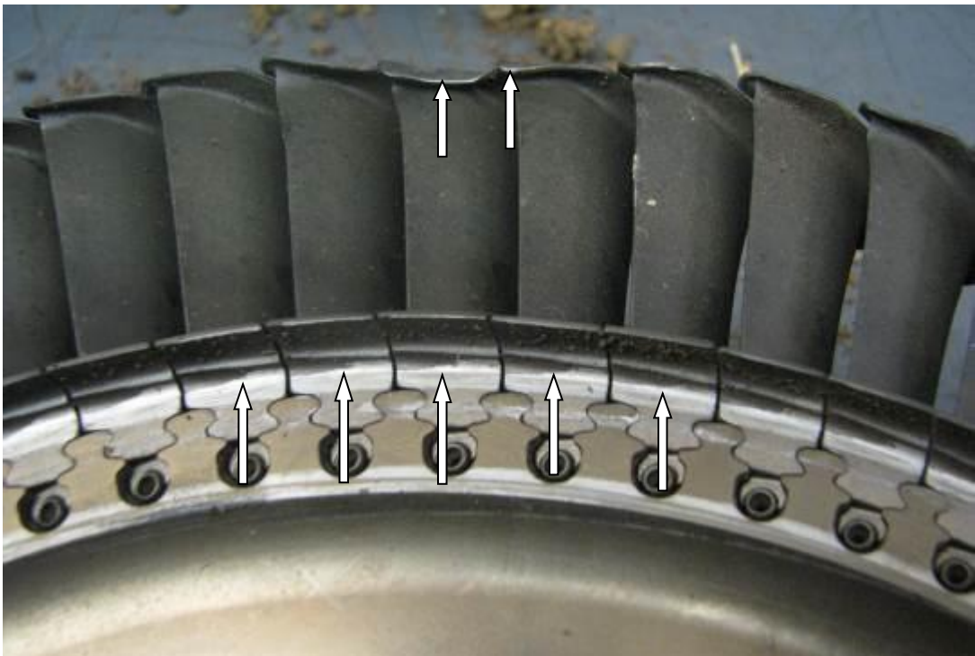
Figure 26: Rub marks on the low-pressure (LP) turbine disk and blades
