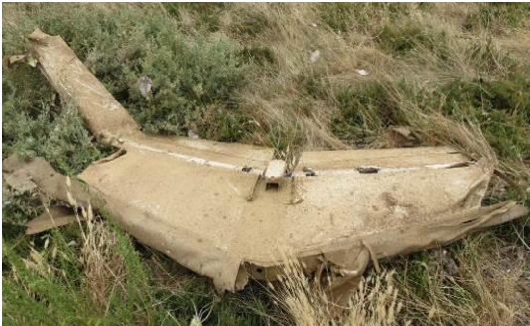
Figure 14: The vertical stabiliser with both elevators attached
