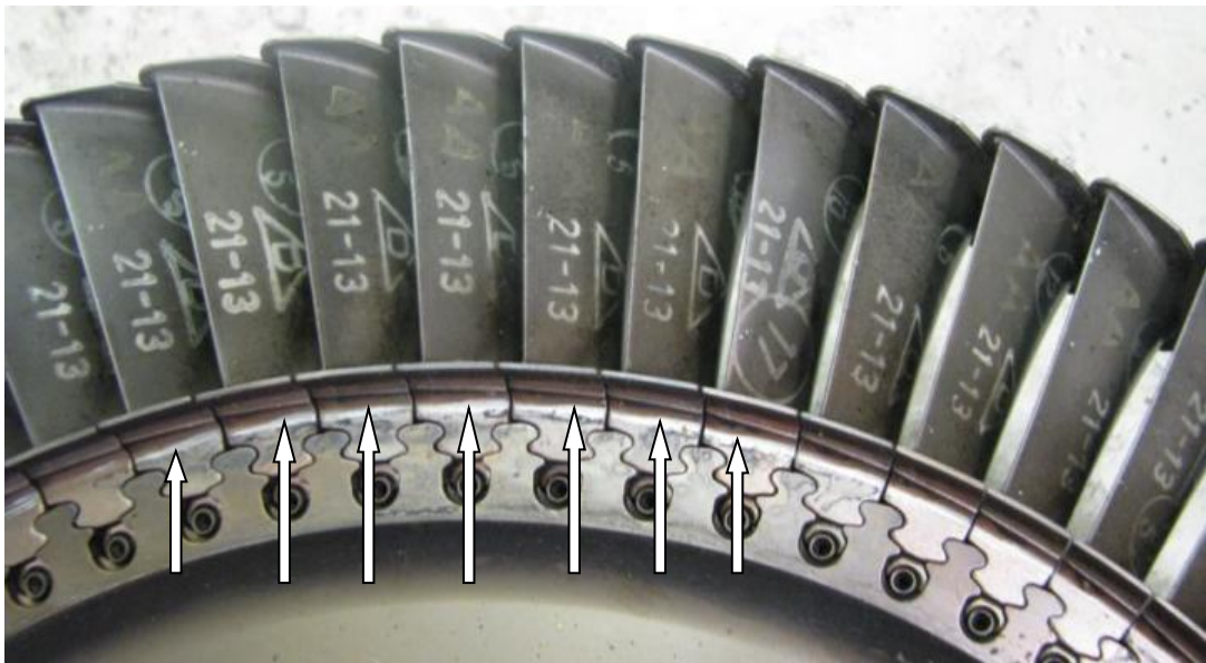
Figure 32: The low-pressure turbine disk with rub marks visible
