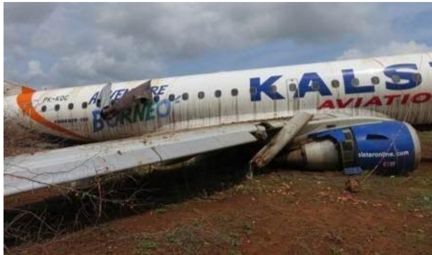
Figure 1: The damaged right wing
