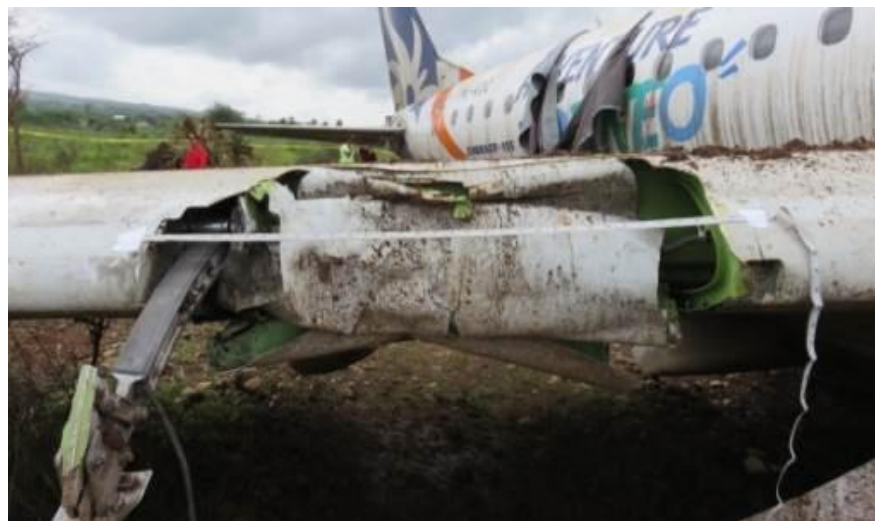
Figure 2: The impact damage on the right wing
