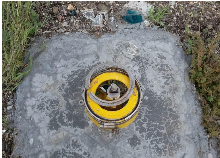
Figure 3: Broken runway light
