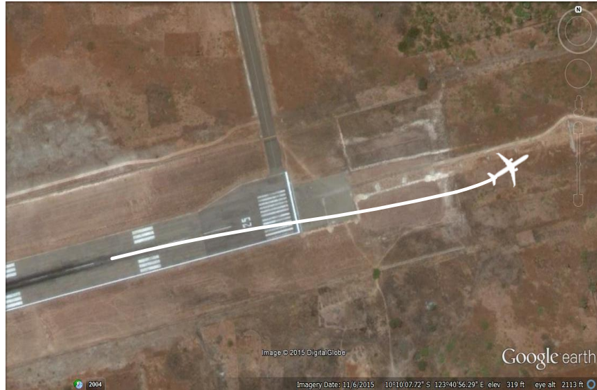
Figure 15: Illustration of tire mark when the aircraft started to veer from runway centerline (white line)
