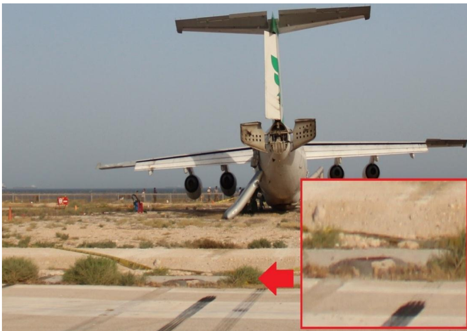
Overrun location and signs of nose impact
