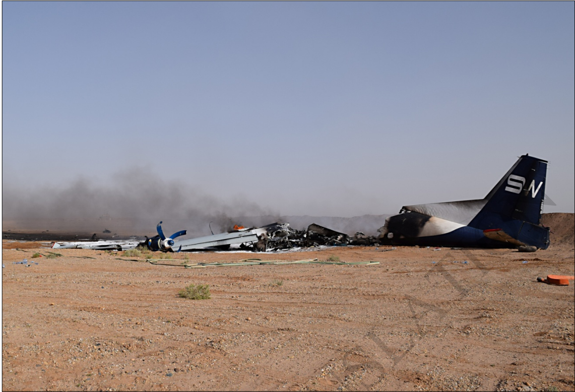
Figure 1. A/c at the accident site destroyed by the post-crash fire
