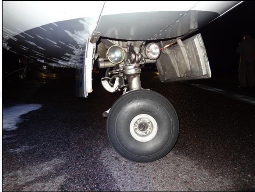
Figure 3 - Damage to the nose landing gear.
