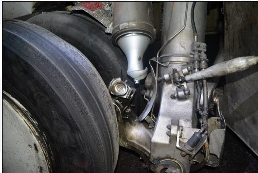
Figure 2 - Damage to the right landing gear.
