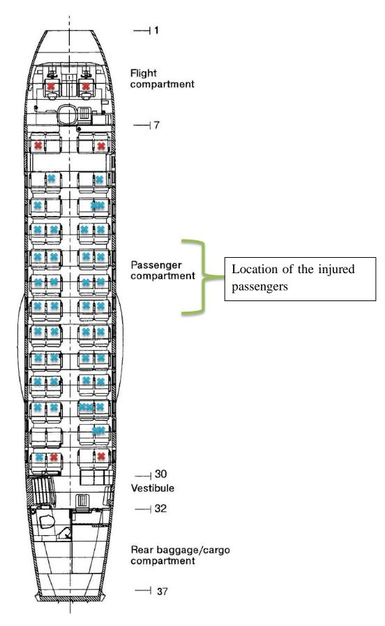
Figure 19: flight deck crew and passenger seats configuration
