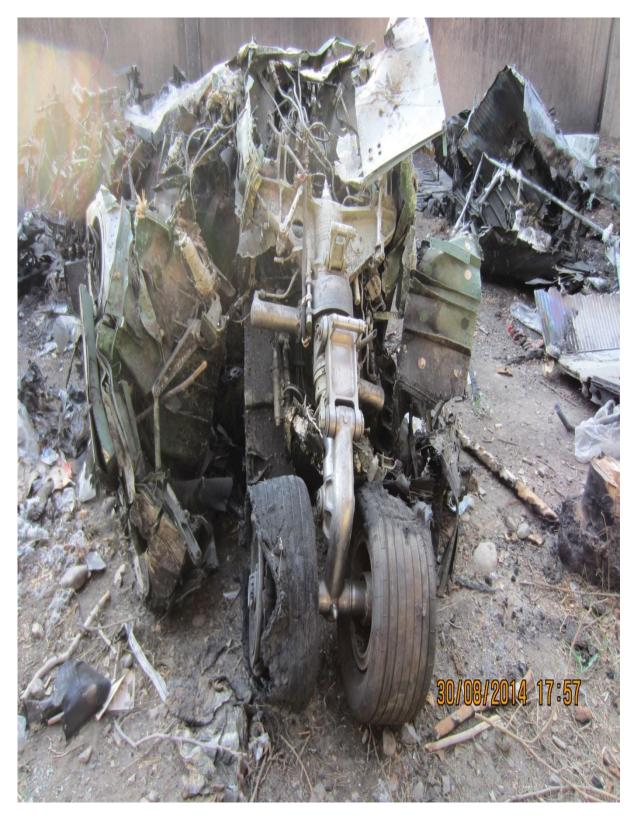
Figure 14. AN-140-100 Wreckage-landing gear
