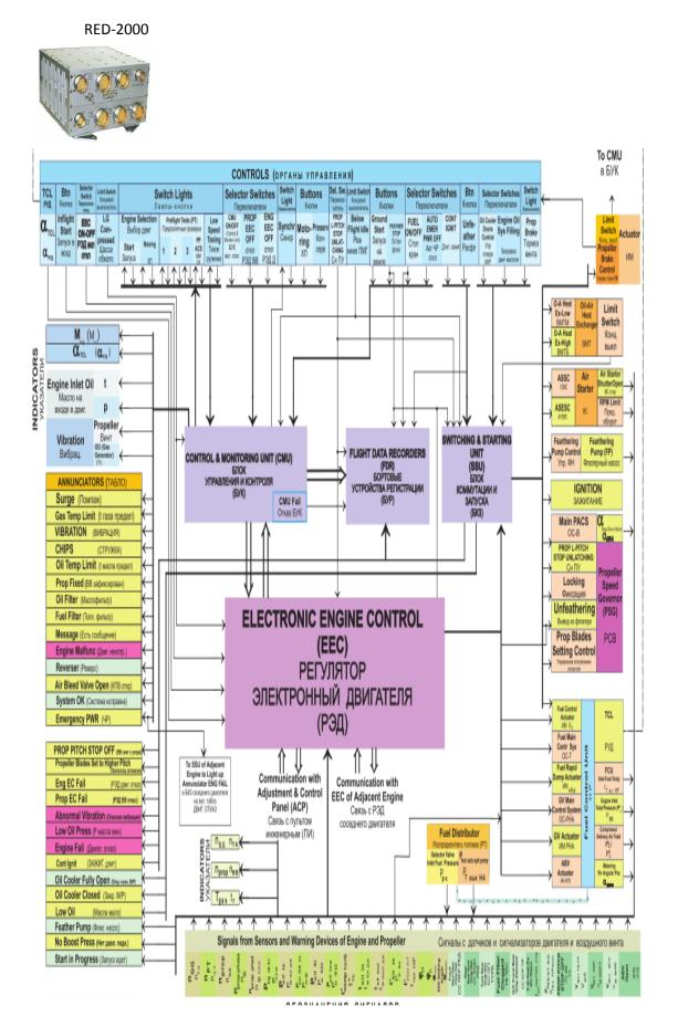
Figure 6: TB3-117BMA-CFM engine and related electronic control diagram.
