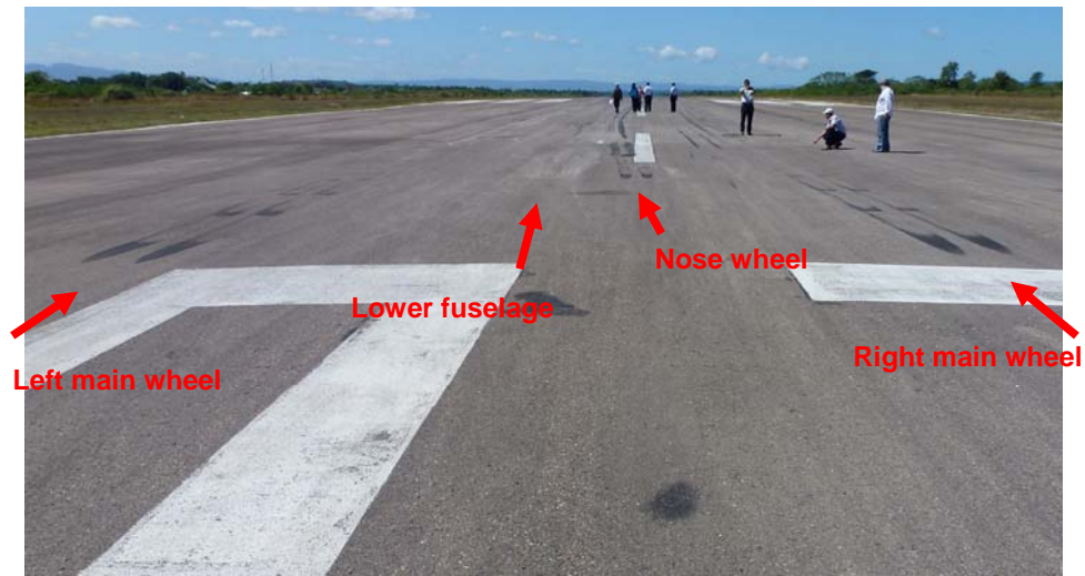
Figure 12: The marks of the initial touch down
