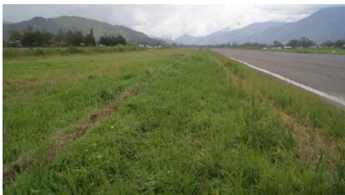
Figure 7: The mark of both main wheels off the runway
