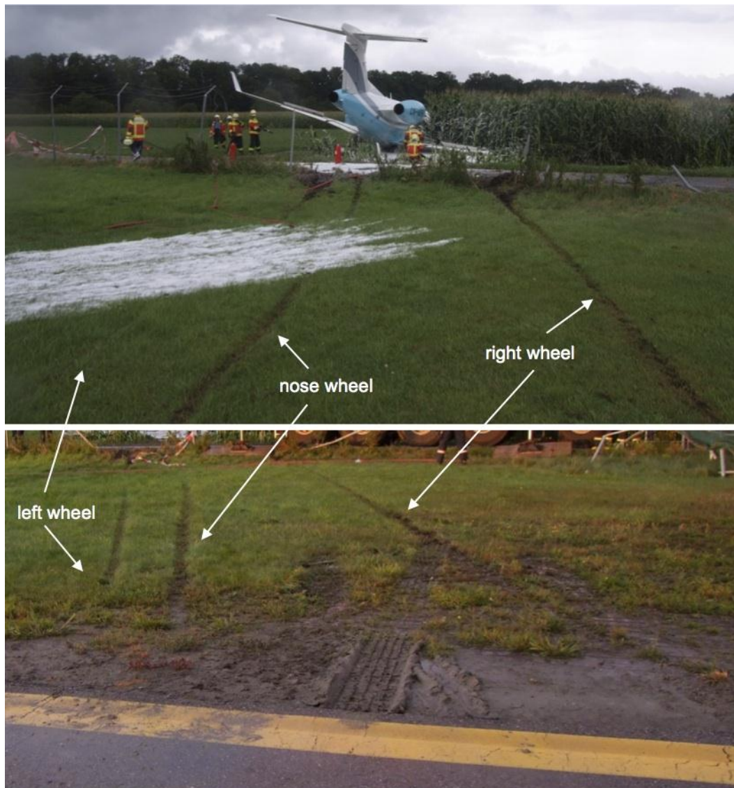
Figure 21: Aircraft wheel marks after it rolled beyond the end of the runway
