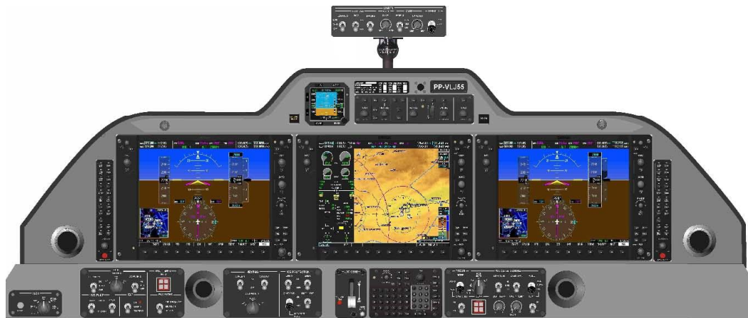
Figure 1: Overview of cockpit front panel with screen selection for normal operation: left and right primary flight display (PFD) and in the centre a multifunction display (MFD)
