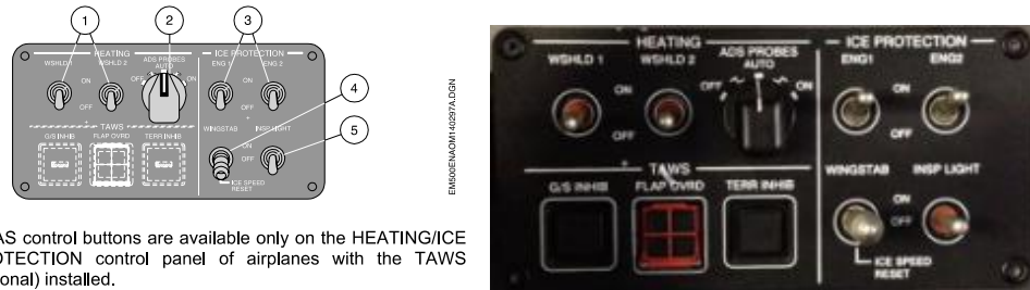
Figure 10: HEATING/ICE PROTECTION control panel (left: POH 2908, 6-11-05; right: in aircraft CN-MBR)
