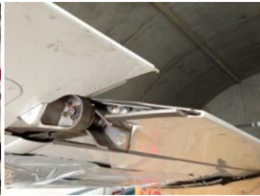
Figure 25: Flaps on left wing, 9.49° extended
