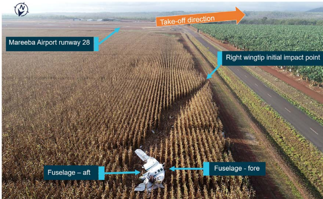
Figure 2: Accident site showing the take-off direction, initial impact point and fuselage resting position
