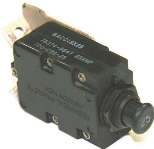
**Figure 8:** BACC18X25 circuit breaker in the “as received” condition.
