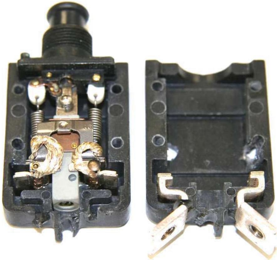
**Figure 15:** BACC18X25 housing open.
