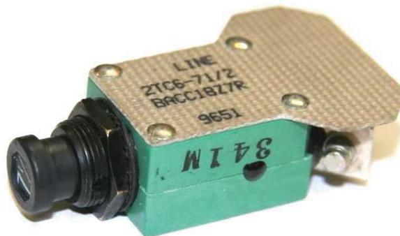
**Figure 7:** BACC18Z7R circuit breaker in the “as received” condition.
