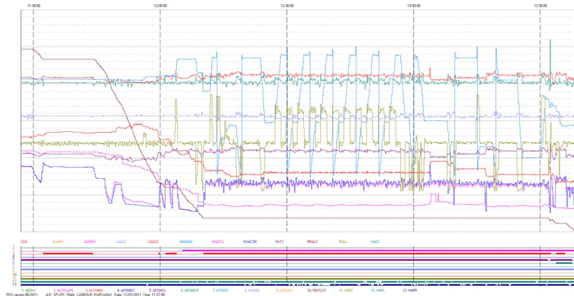
Figure 14. SP-LPC approach to landing – as recorded by the SSFDR.
