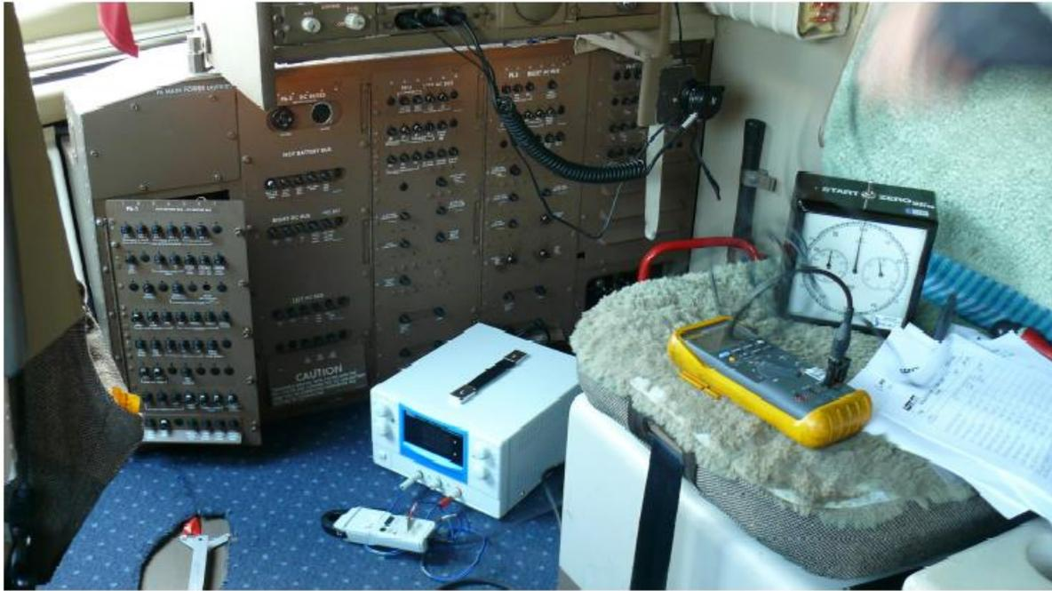
Fig. 17. Test set for measurement of the trip time of the circuit breakers
