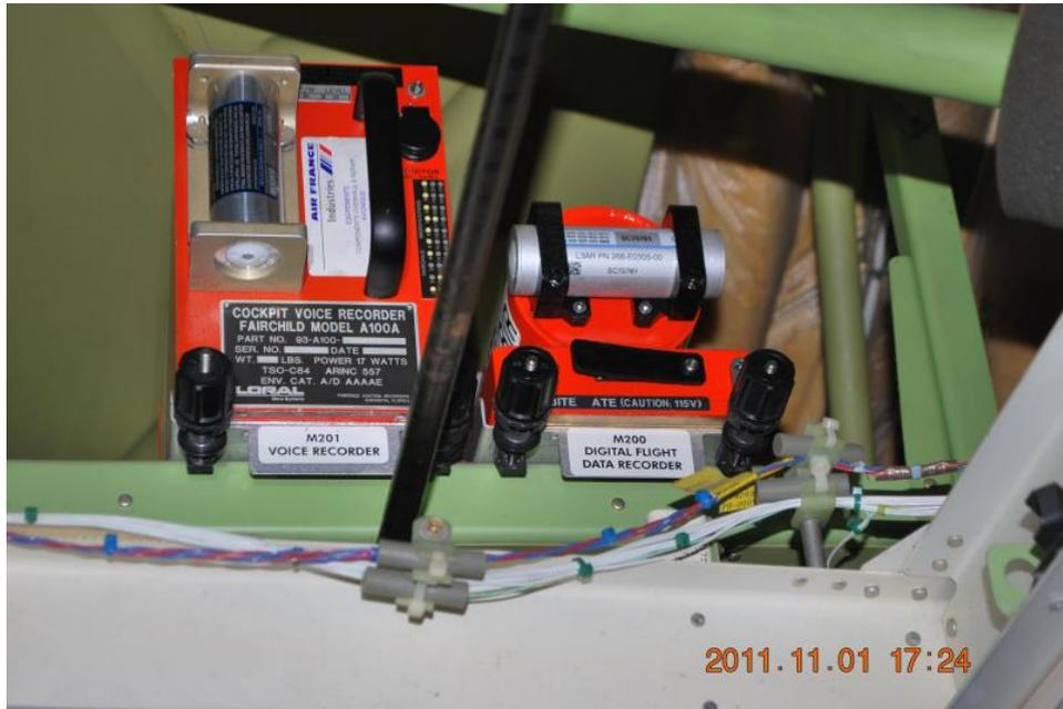
Figure 8. CVR and SSFDR removed from SP-LPC airplane. (Source: SCAAI)
