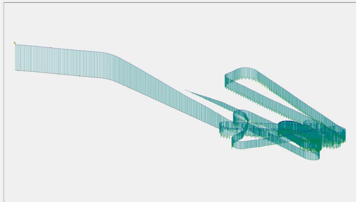
Figure 11. 3-D view of the LO 16 flight path during holding in the area of EPWA.
