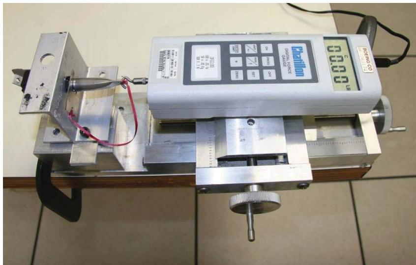
Figure 12: Operating force test setup.
