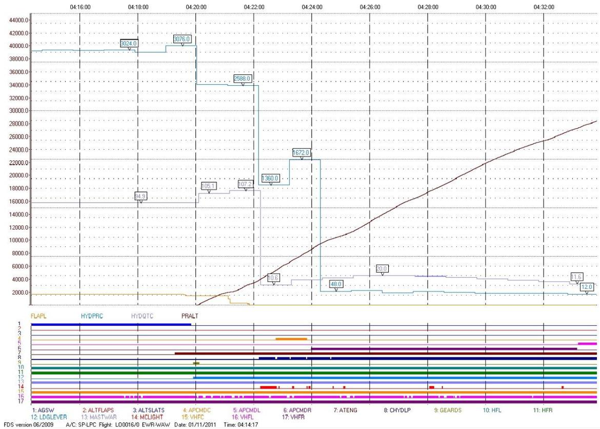
Figure 13. Pressure drop in the center hydraulic system of SP-LPC after its take-off - as recorded by the SSFDR.
