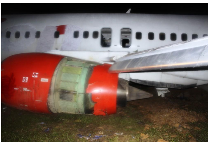
Figure 1: The damage of the left engine
