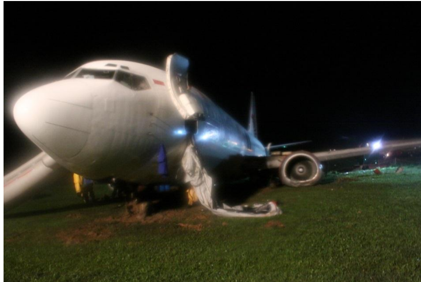
Figure 7: The front left escape slide flattened
