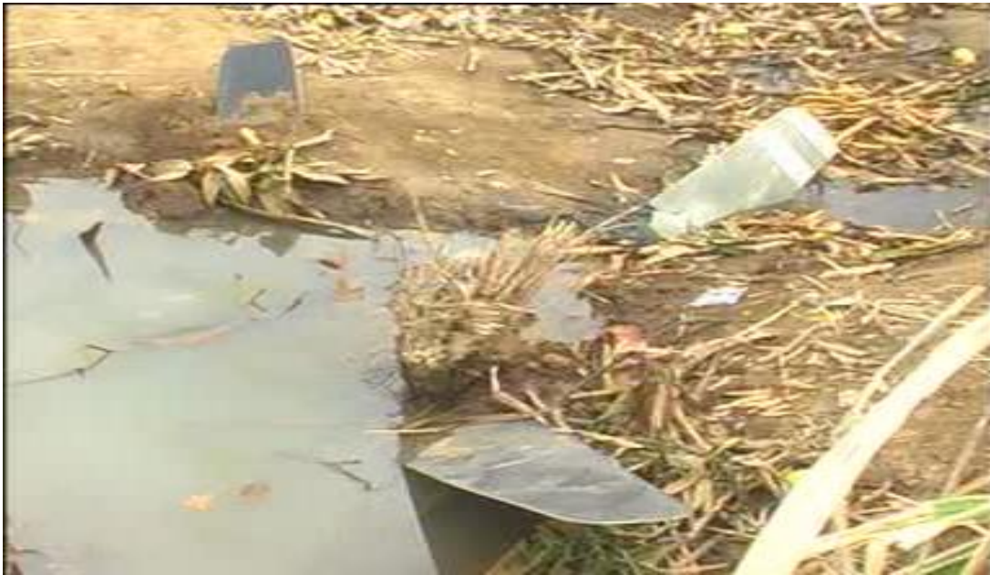
Figure 5: Detached right propeller blade assembly
