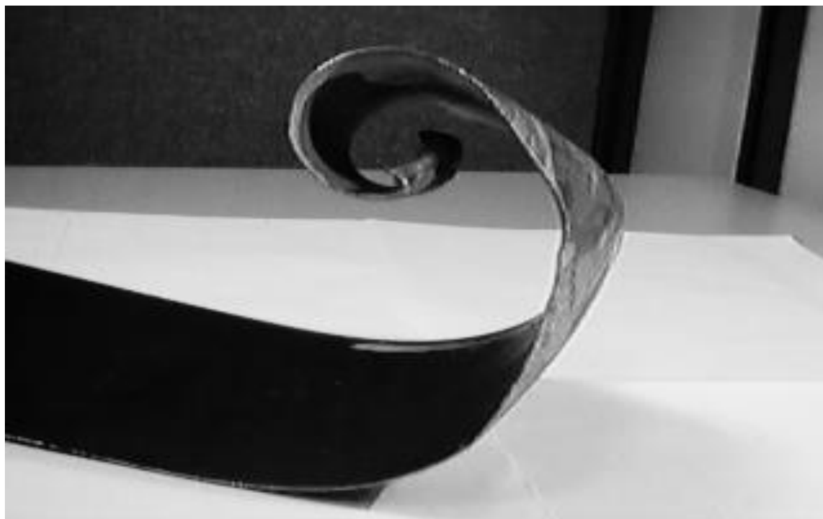
Figure III-12-35. Propeller tip bent forward as a result of high rpm during a low-angle impact
