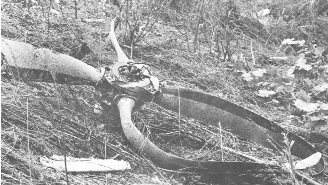
Figure III-12-31. Metal propeller under power at impact
