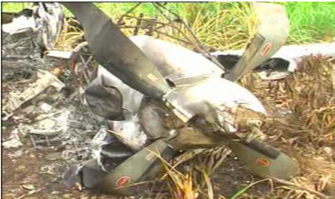
Figure 6: Left engine propeller blades bent backward
