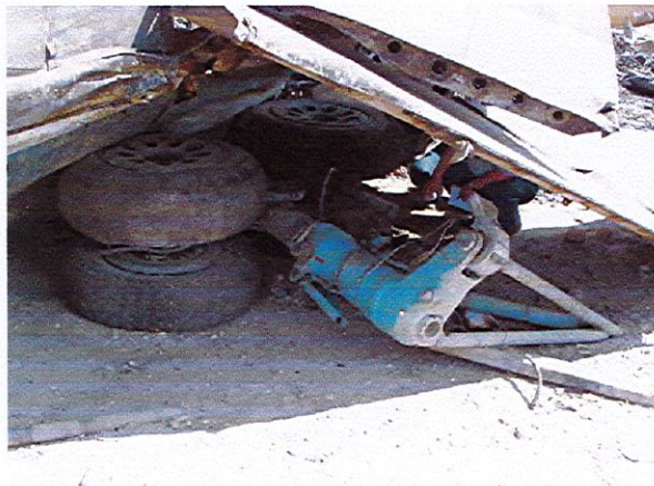
Right main L/G found 50 meters away from the wreckage and partially destroyed.
