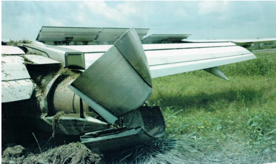
Figure 2: The number 2 engine thrust reverser damage.
