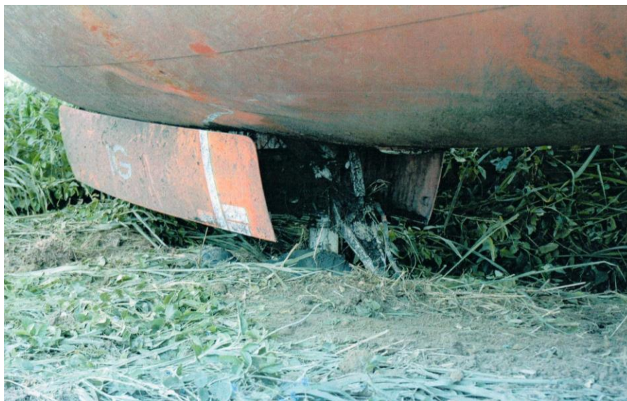
Figure 3: Damaged nose wheel gear
