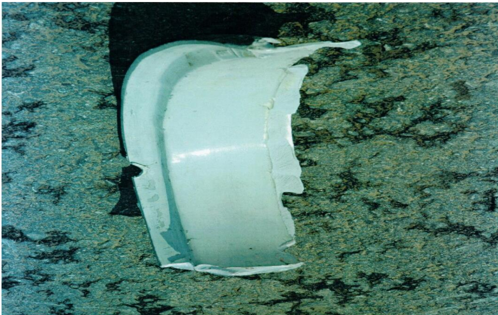
Figure 7: Another broken piece of the nose wheel rim
