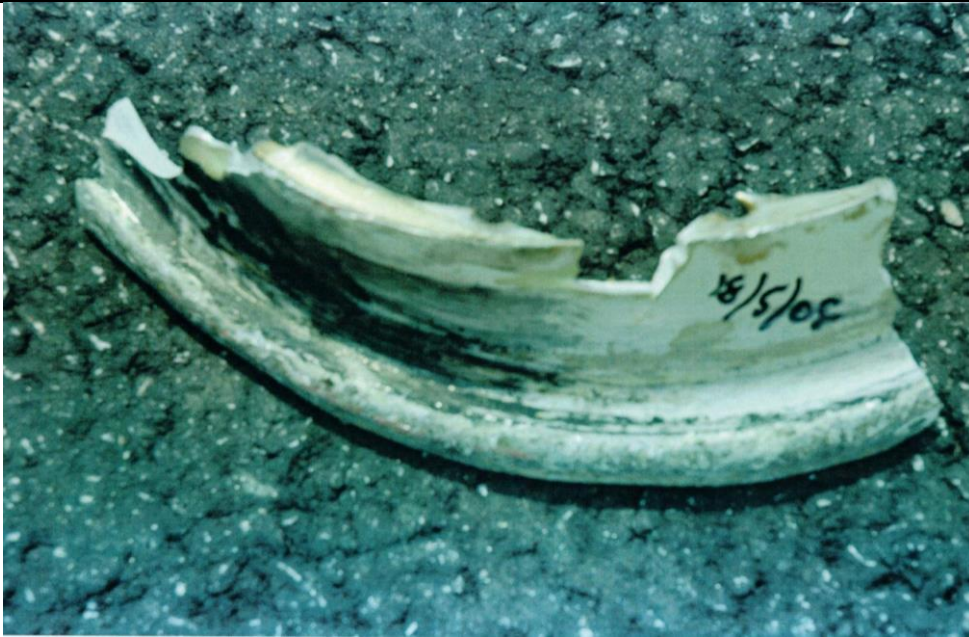
Figure 6: A broken piece of the nose wheel rim
