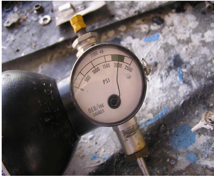
Emergency gear blow down bottle showing a positive pressure charge on the nitrogen bottle.
