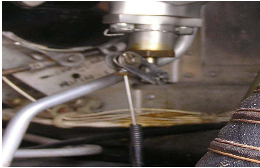
Emergency gear extension system cable prior to selector handle being pull to activate system.
