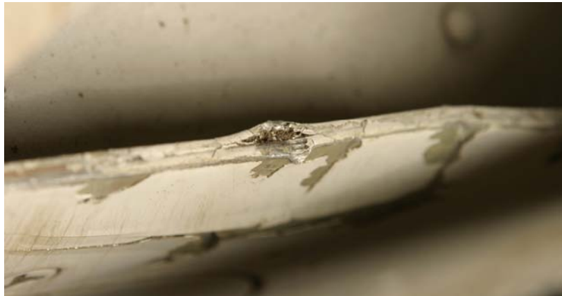
Damage to shell plating on underside of wing
