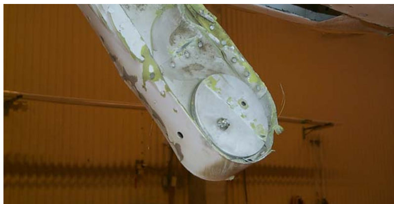
Broken fixing bolt for balance weights
