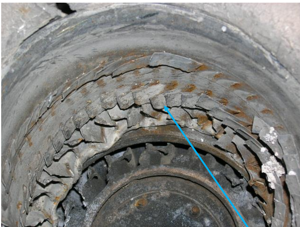
Figure 11 Compressor stator vanes and shrouds, and centrifugal impeller, lower circumference
