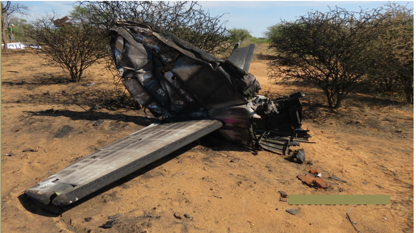
Figure 4. Photo showing the broken off empennage
