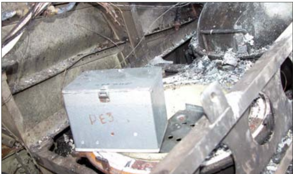
FIGURE 15: Cockpit voice recorders during recovery from the aircraft wreckage
