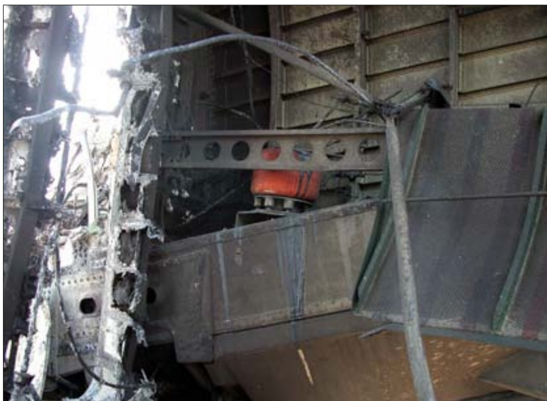
FIGURE 13: Flight data recorder before recovery from the aircraft wreckage
