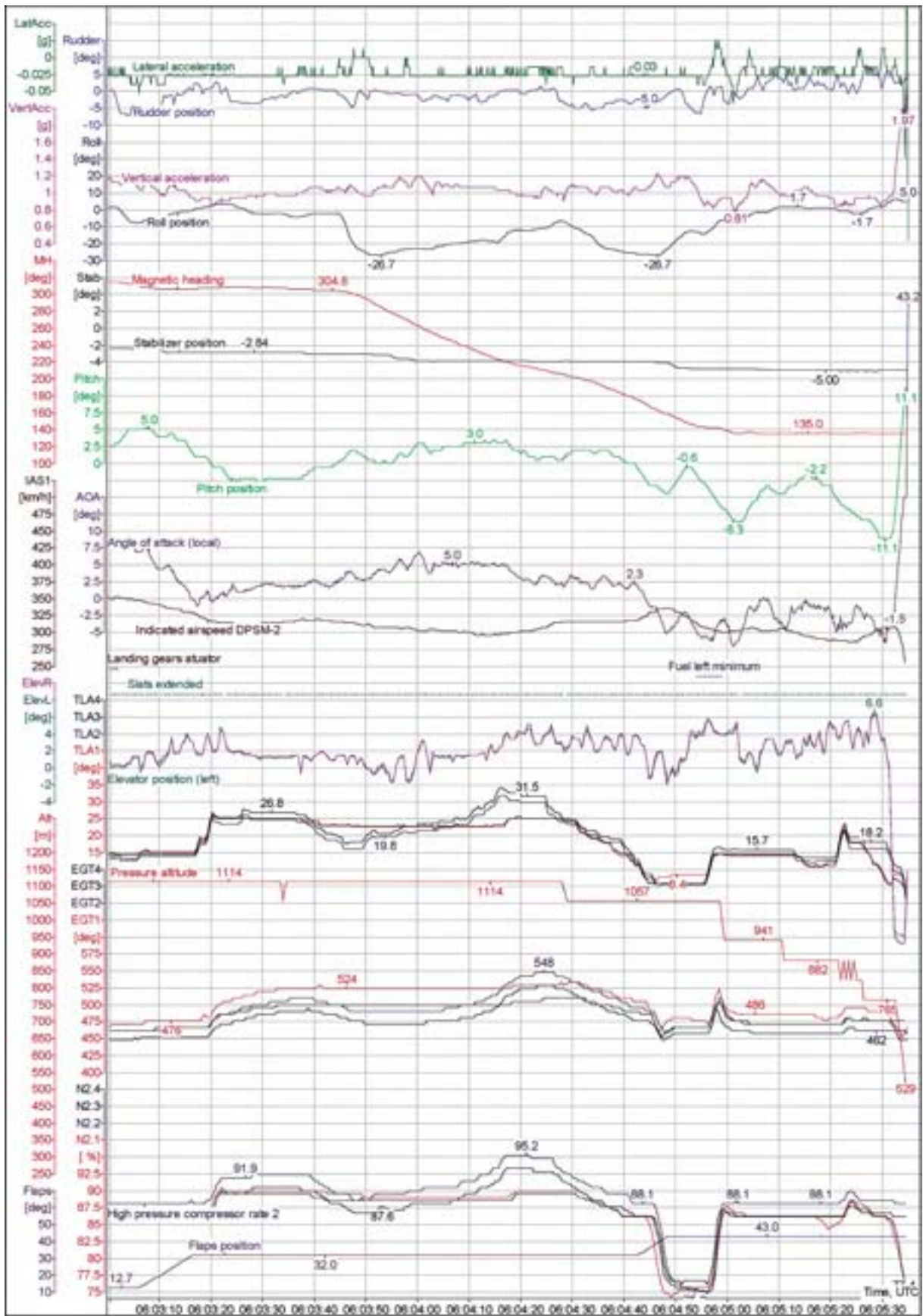
FIGURE A.9: FDR data plots for the final landing approach at Baucau
