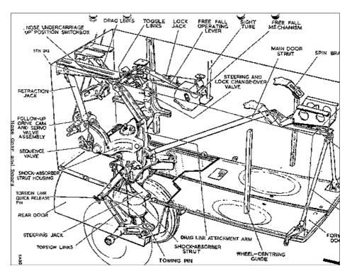
Time between overhauls of the nose gear is 11 years or 15 000 cycles. It was overhauled by the manufacturer, BAe in England, on 31 January 1993 and had since accumulated 2 224 hours and 2 064 cycles.
